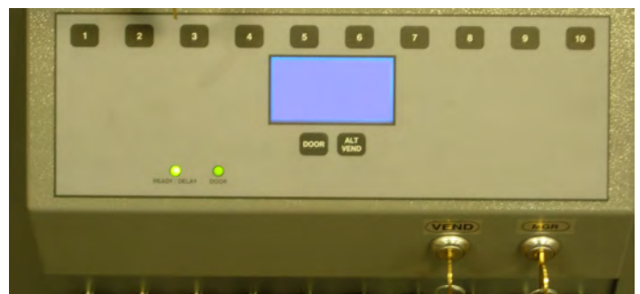
Keypad Membrane MGR Key Switch (far right) VEND Key Switch (to the left)
