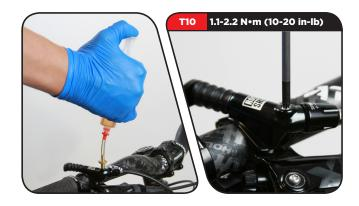
Depress the remote actuator five times. Release it to allow the actuator to return to its extended position.
