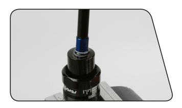
Thread the inner seal head into the upper post to completely install the inner shaft piston into the IFP tube.
