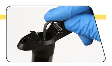
4 Use a Schrader valve tool to remove the Schrader valve from the upper post.
