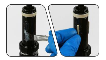
Slide the lower post over the upper post and onto the inner seal head. Squeeze the inner seal head bushing, then slide the lower post down and over the seal head bushing. Align the lower post with the brass keys and ensure the laser etched RockShox logo is lined up with the back of the seat post head.
