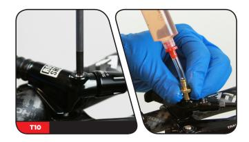
Use a T10 TORX® to remove the bleed screw from the bottom of the seatpost, then install the empty syringe into the bleed port.
