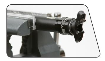
Use a 34 mm open end wrench to unthread the top cap assembly from the lower post.
