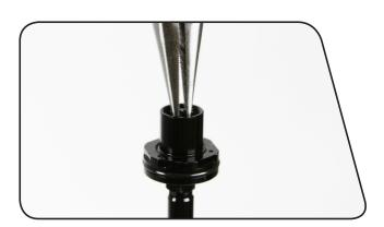
Hold the seal head in place with an 11 mm open end wrench. Thread the poppet valve cover onto the seal head, then use a 10 mm crowfoot socket to tighten the poppet valve cover to 5.7-7.9 N•m (50-70 in-lb). Install the crowfoot socket at 90 degrees to the torque wrench.
