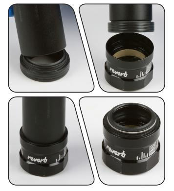
Use your fingers to remove the o-rings from the seal head. Clean any dirt or debris from the seal head, and install new o-rings.
