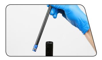
Remove the top cap assembly from the upper post.
