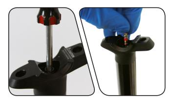
Use a Schrader valve tool to install a new Schrader valve into the air fill valve.
