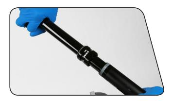
Use internal snap ring pliers to reinstall the snap ring. Check that the snap ring is securely installed in the groove by using the snap ring pliers to rotate it in the groove.
