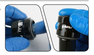
Install the IFP tube with cross holes facing up into the upper post. Push down firmly on the IFP tube until it snaps securely into the upper post. Ensure the IFP tube is secured and centered. The IFP tube should be below the top of the upper post when installed correctly.
