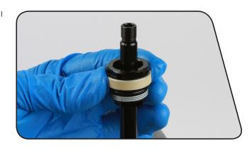
6 Insert the end of the inner shaft piston into the IFP tube just enough for the piston o-ring to engage the IFP tube.
