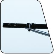
Use your fingers to remove the two backup rings and the o-ring from the inner shaft piston. Clean the inner shaft piston and install two new backup rings and a new o-ring. The o-ring must be located between the backup rings.
