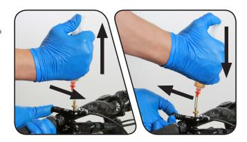
Depress the remote syringe plunger and make sure the remote actuator is fully extended. Remove the syringe and use a T10 TORX® to reinstall the bleed screw and tighten to 1.1-2.2 N•m (10-20 in-lb).
