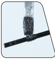
Insert the poppet valve into the inner shaft, then use needle nose pliers to press it firmly into the seal head.
