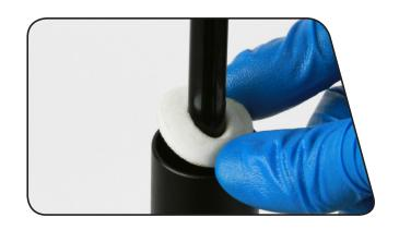
Clamp the inner shaft in a vise with soft jaws. Thread the seal head onto the inner shaft, then use an 11 mm crowfoot socket to tighten the seal head to 5.7-7.9 N•m (50-70 in-lb). Install the crowfoot socket at 90 degrees to the torque wrench.
