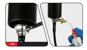
Depress the remote syringe plunger while pulling out on the seatpost syringe plunger. Depress the plunger of the syringe attached to the seatpost while pulling out on the remote syringe plunger.
