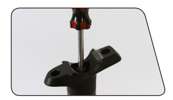
Open the seatpost clamp or loosen the seatpost collar binder bolt and remove the Reverb Stealth from the bicycle. It is not necessary to remove the Reverb remote from the handlebar unless the remote housing is too short to allow the Reverb to be removed from the frame.
