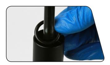
355 & 420 mm Reverb Stealth with 100 mm travel, and 420 mm Reverb Stealth with 125 mm travel: Apply SRAM Butter to the false bottom insert o-ring, then install it into the lower post. Orientation of the false bottom insert is not critical.
