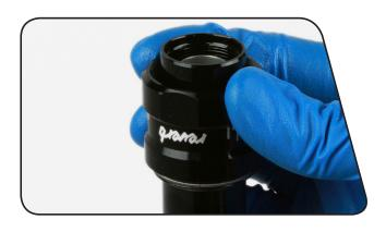
Insert a 1.5 mm hex wrench into one of the cross holes of the IFP tube. Use pliers to carefully pull the IFP tube out of the upper post.
