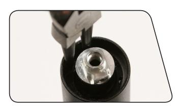
Clamp the lower post in a vise. Use a 34 mm crowfoot socket to tighten the top cap to 27-29 N•m (238-256 in-lb). Install the crowfoot socket at 90 degrees to the torque wrench.
