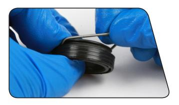
Insert the small end of the new dust wiper into the end of the lower post. Orient the top cap on the bench with the logo facing up, and use the lower post to press the dust wiper into the top cap. Reinstall the energizer ring.
