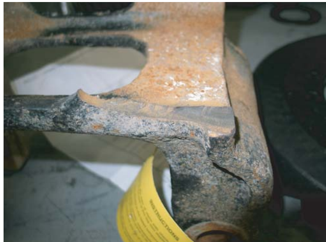
Hanger Bracket Fatigue
