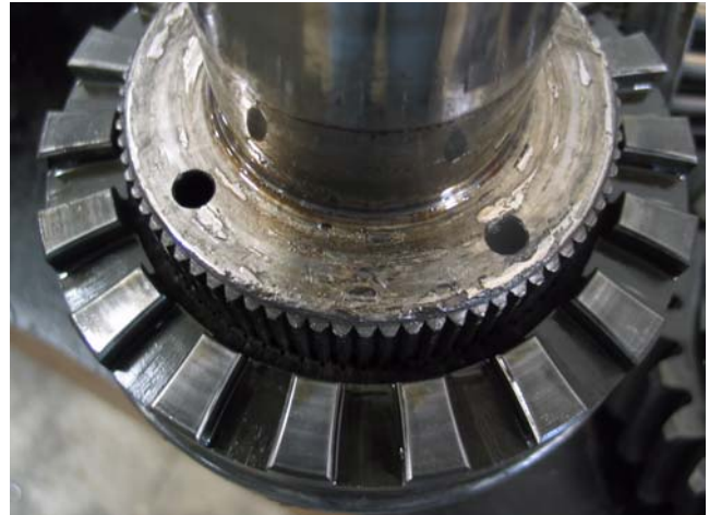
Input Shaft Stub-End - Galling
