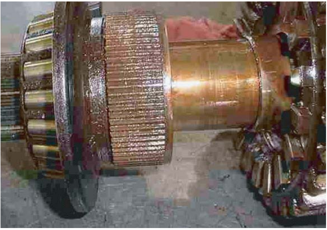
Input Shaft Stub End - Water Contamination
