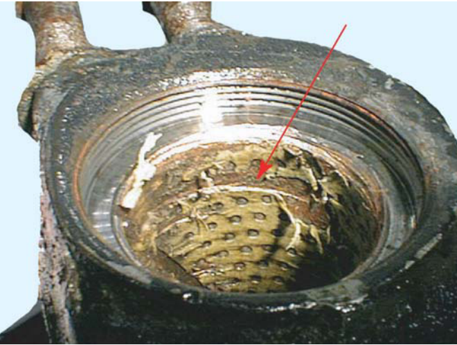
Improper Kingpin Installation
