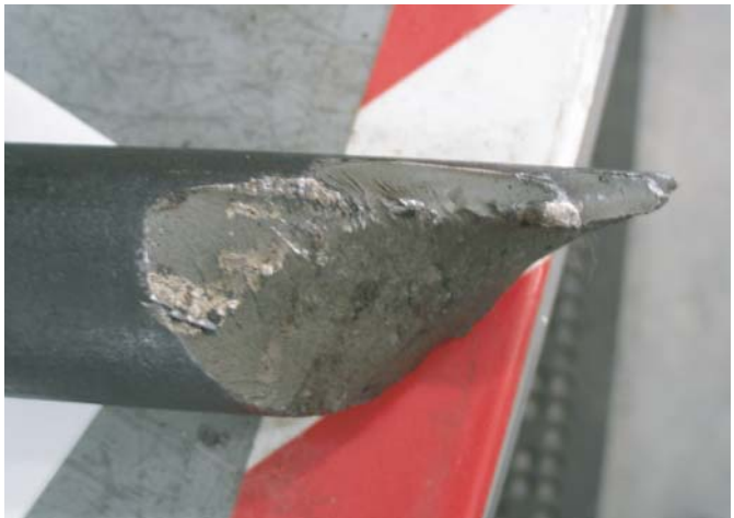
Axle Shaft - Shock
