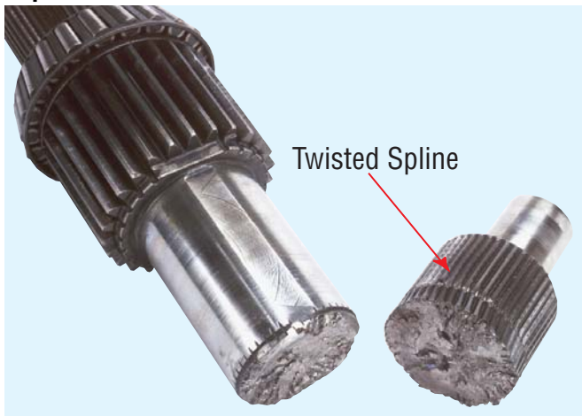
Input Shaft - Torsional Shock Failure
