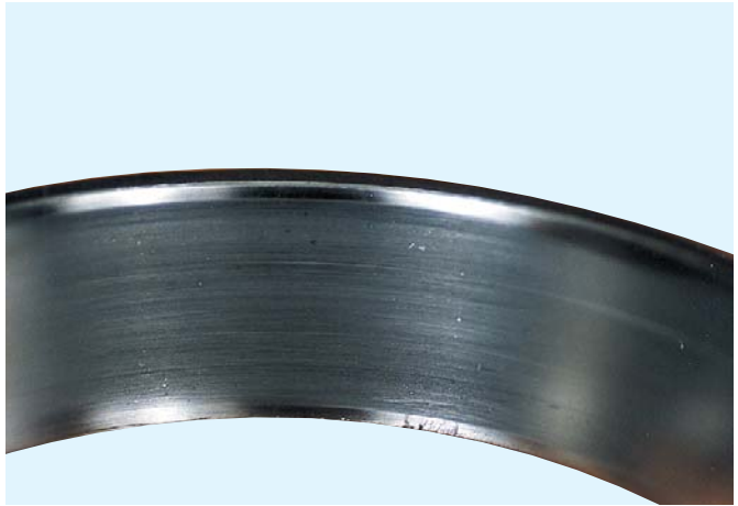
Contamination - Bruising (Denting)
