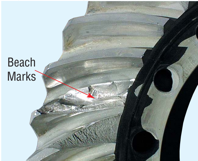
Drive Pinion - Torsional Fatigue Failure
