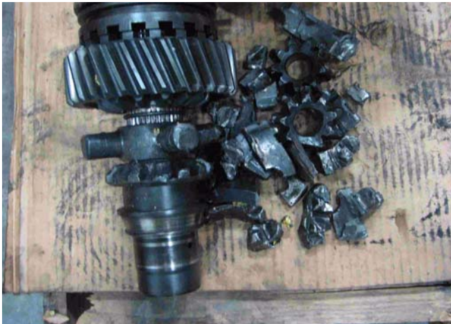
Input Shaft Assembly - Catastrophic
