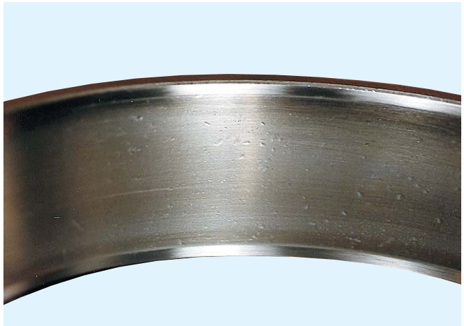
Contamination - Bruising (Denting)
