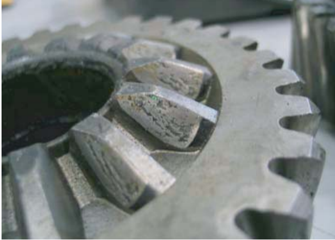
Output Side Gear - Spalling
