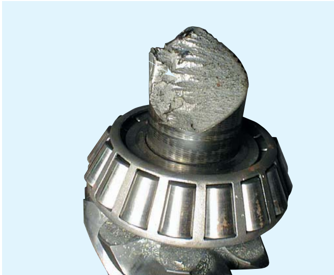
Drive Pinion - Torsional Shock Failure
