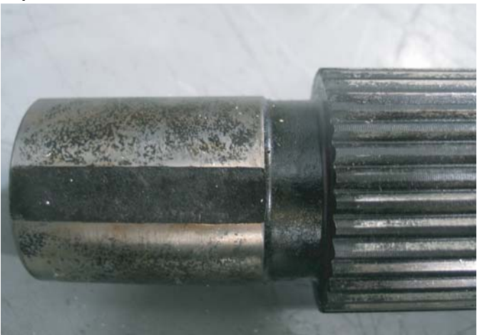
Input Shaft Stub End - Water Contamination
