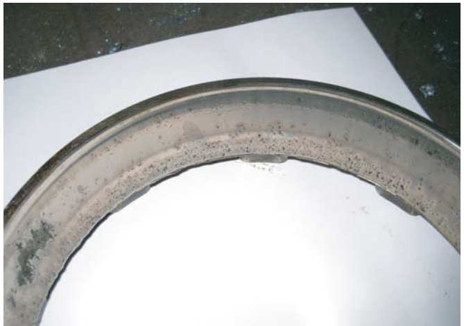
Bearing Cup - Water Contamination
