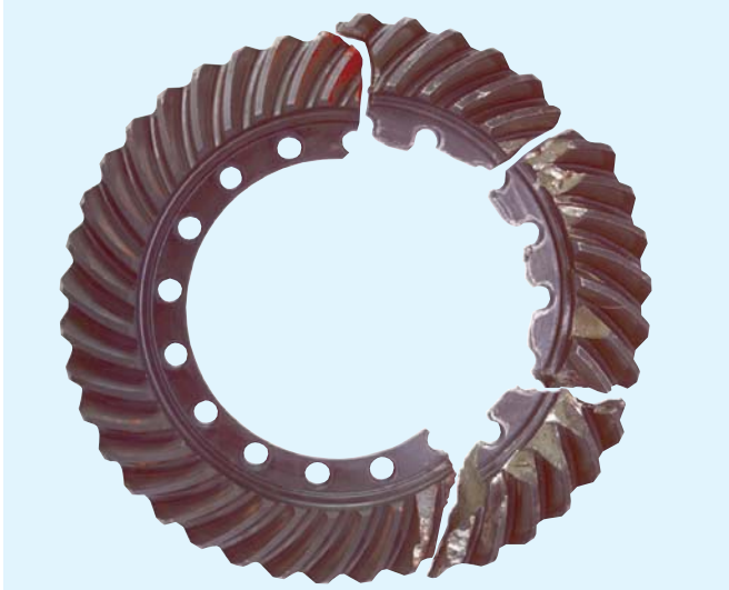
Drive Pinion - Torsional Shock Failure
