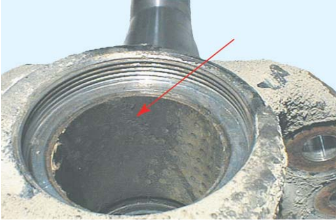
Bushing - Lack of Grease
