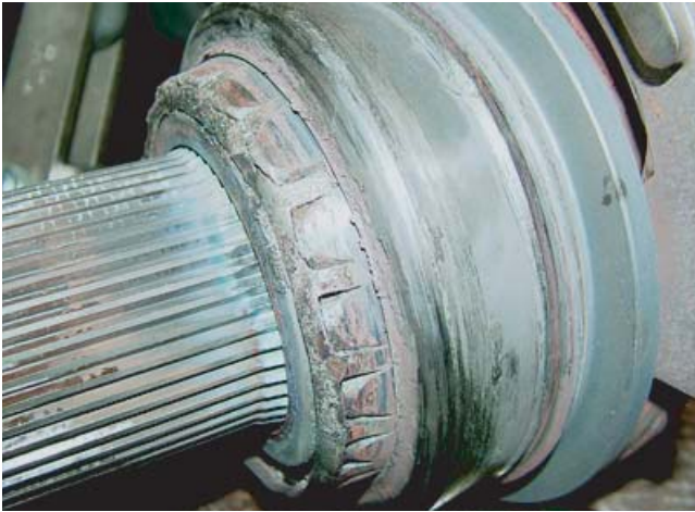
Helical Side Gear Bushing - Lubricant Contamination
