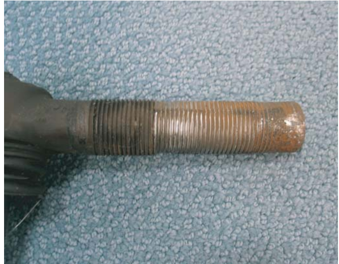
Thread Damage - Loose Clamp Assembly
