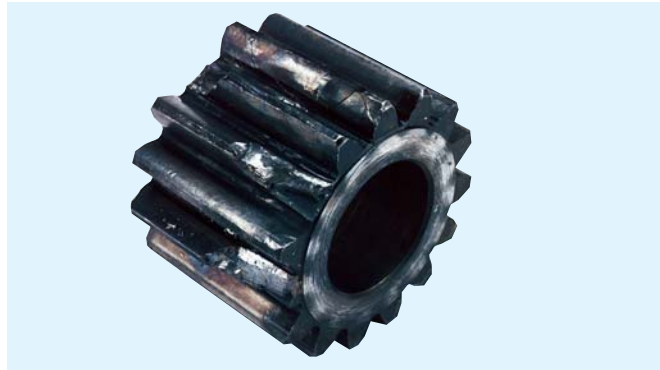
Planetary Gear - Shock Failure
