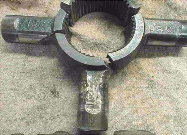
IAD Spider Arm - Bore Galling
