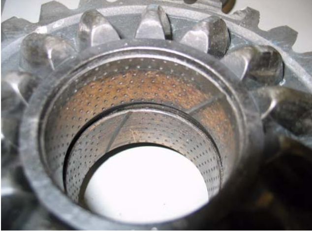
Helical Side Gear Bearing Damage
