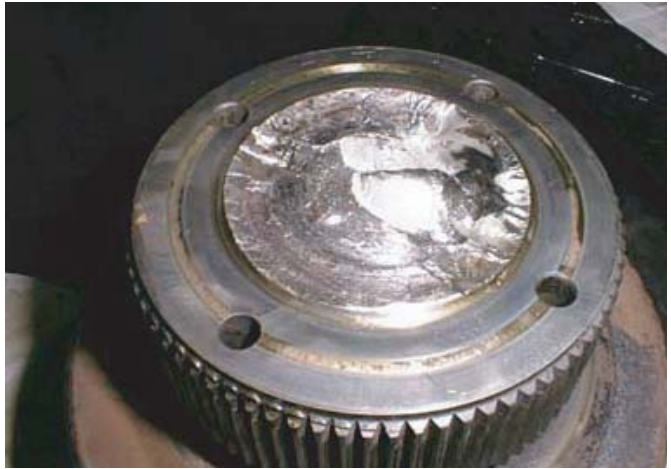
IAD Spider - Fatigue Failure
