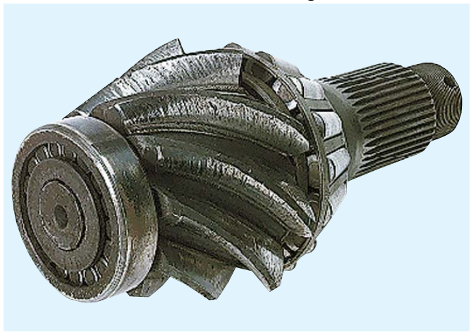
Drive Pinion - Low Lube - Scoring
