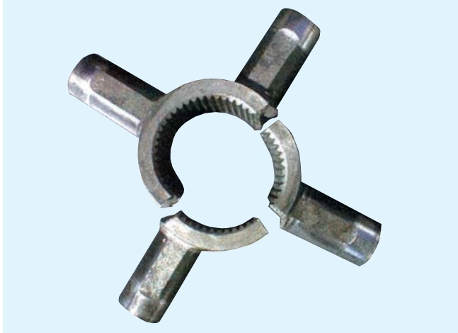
Sliding Clutch - Shock Failure
