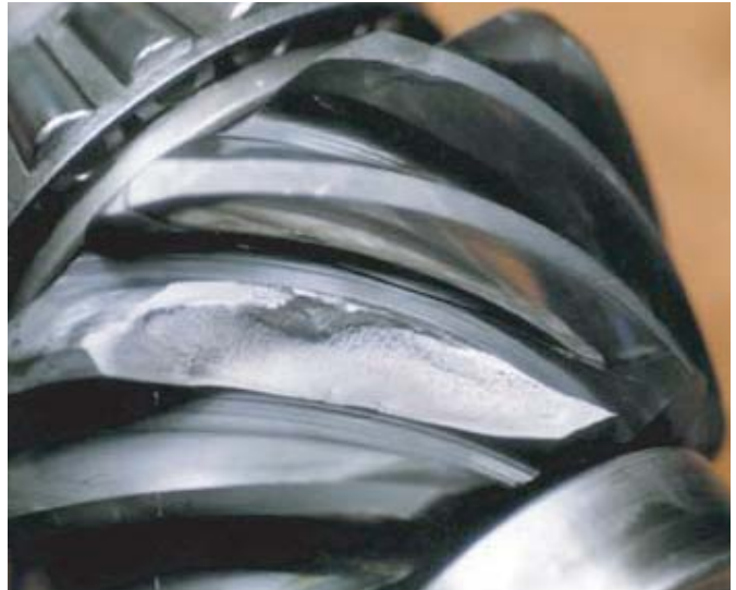
Drive Pinion - Tooth Shock Load Failure
