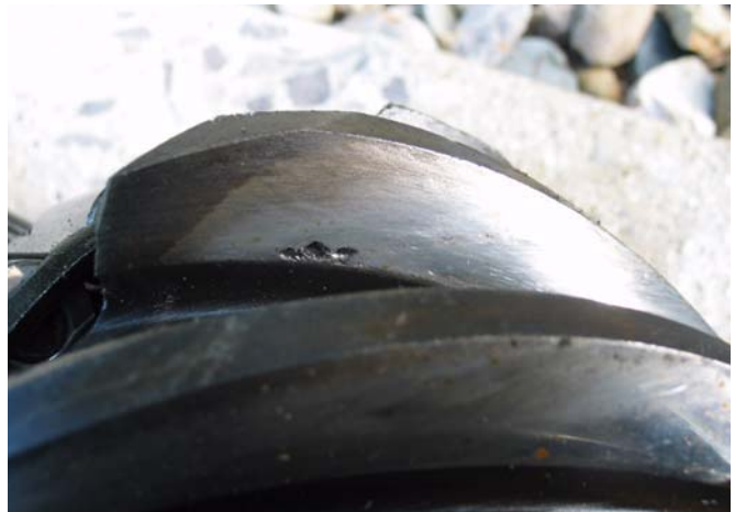
Drive Pinion - Spalling
