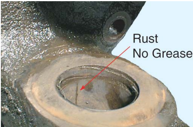
Bushing - Lack of Grease
