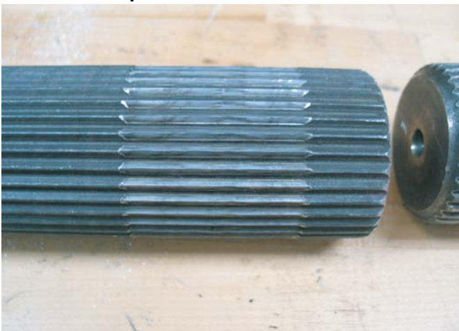
Axle Shaft - Spline Wear
