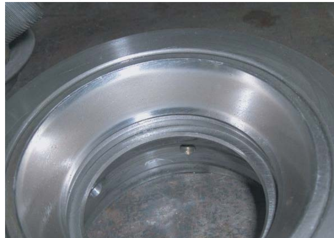
Bearing Cup - Water Contamination
