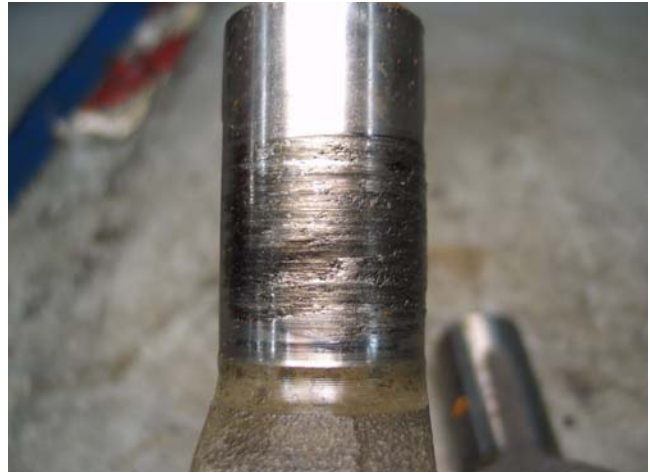
Thrust Washer to Input Shaft - Galling
