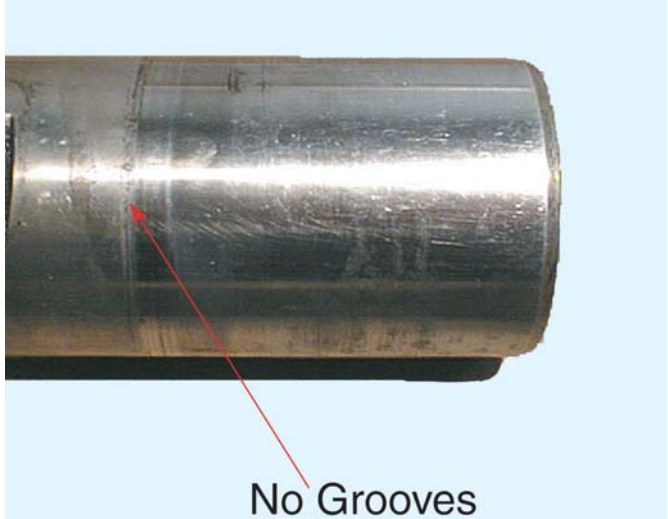
Thread Damage - Loose Clamp Assembly
