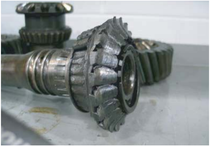
Helical Side Gear Bushing - Water Contamination
