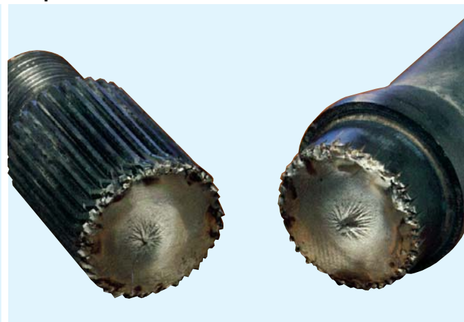
Output Shaft - Torsional Shock Failure
