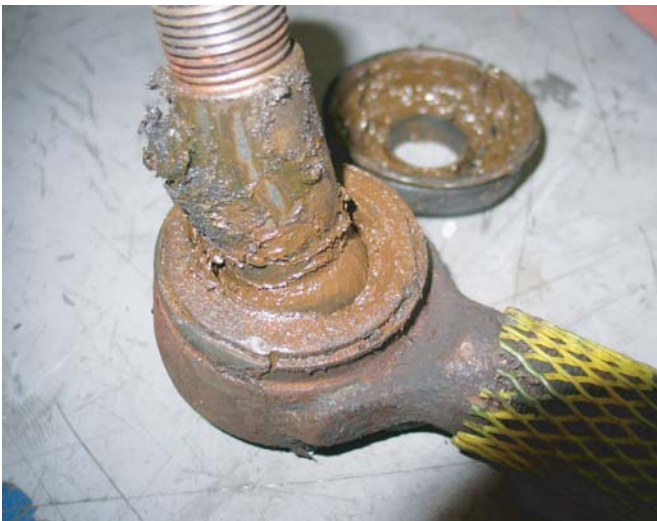
Tie Rod End - Water Contamination
