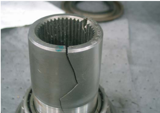
Output Side Gear - Shock
