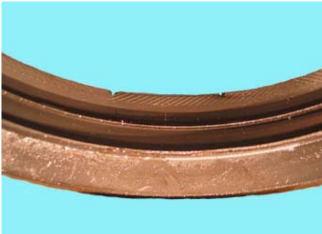
Damaged Seal Lip
