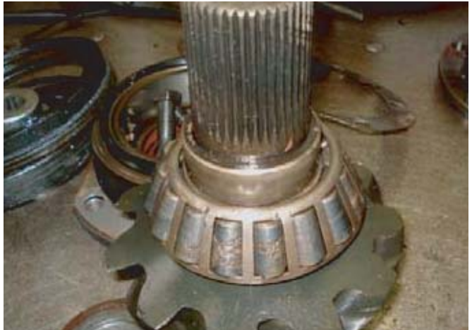
Bearing Cup - Water Contamination
