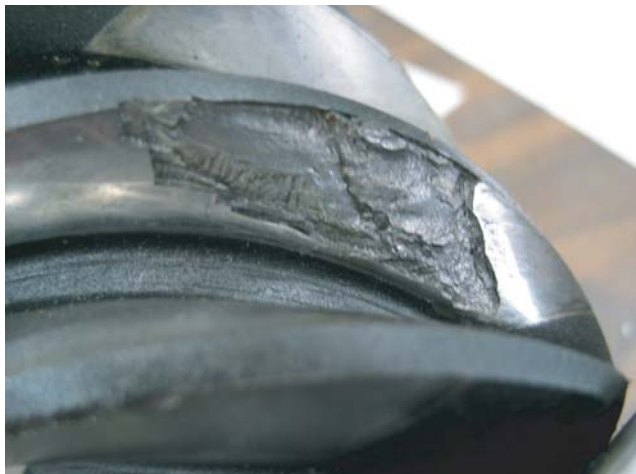
Drive Pinion - Case Crush
