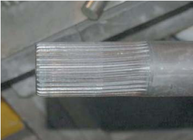
Axle Shaft - Torsional Fatigue Failure
