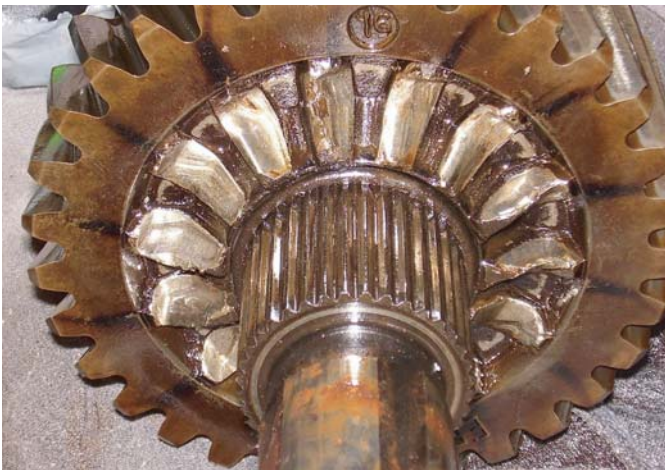
Helical Side Gear Wear - Water Contamination
