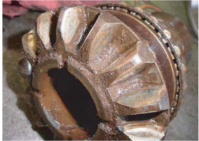
Output Side Gear - Water Contamination
