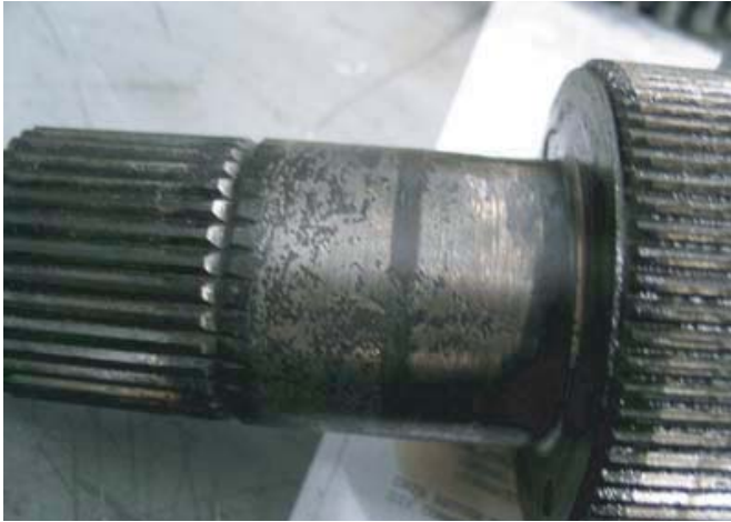
Input Shaft Stub End - Water Contamination
