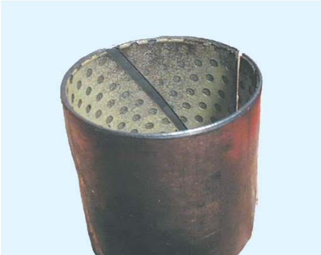
Tie Rod End - Water Contamination
