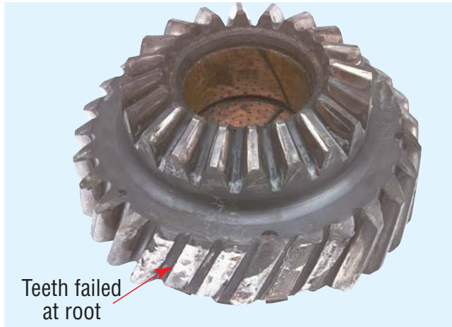
Input Shaft - Torsional Shock Failure
