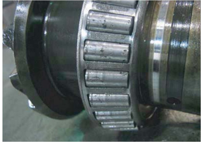
Bearing Cone - Spalling - Water Contamination
