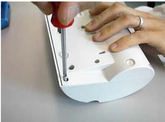
A photograph showing a person's hands using a red-handled screwdriver to remove a screw from the printer's upper housing. The housing is held in a way that allows for easy access to the screws.        |
