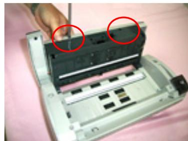
Remove 2 fixing screws
