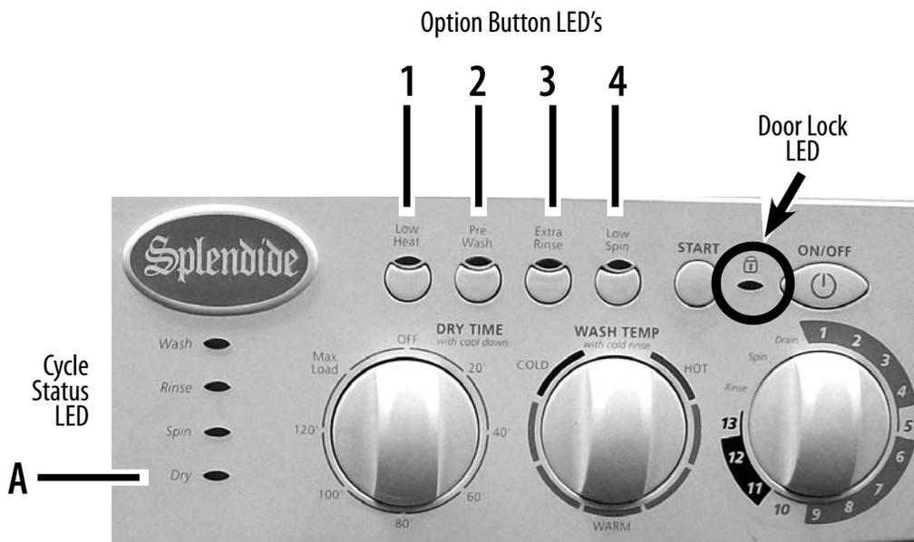
Control Panel Fault Code Display, Fig. 6-1
