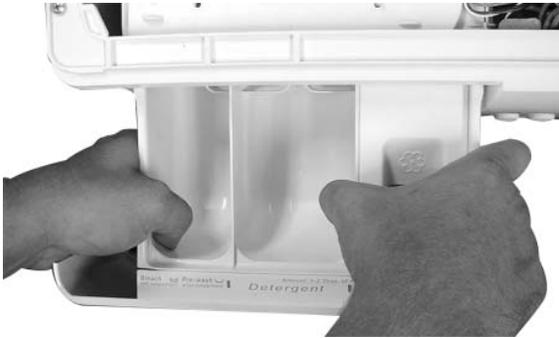
Remove the three Phillips Head screws securing the front of the detergent dispenser assembly to the front of the Control Panel. (Fig. 4-11) Remove the two screws securing the detergent dispenser assembly to the dispenser valves. (Fig. 4-12) Disconnect the two wires from the hot valve.
