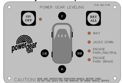
Manual system touch pad #140-1179
