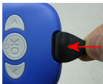
Insert the free end into the Zmachine Sensor/Charger Port
