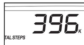
The lower left corner of the display will show the total number of hours that the treadmill has been used and the total number of miles (or kilometers) that the walking belt has moved, for a few seconds at a time.
