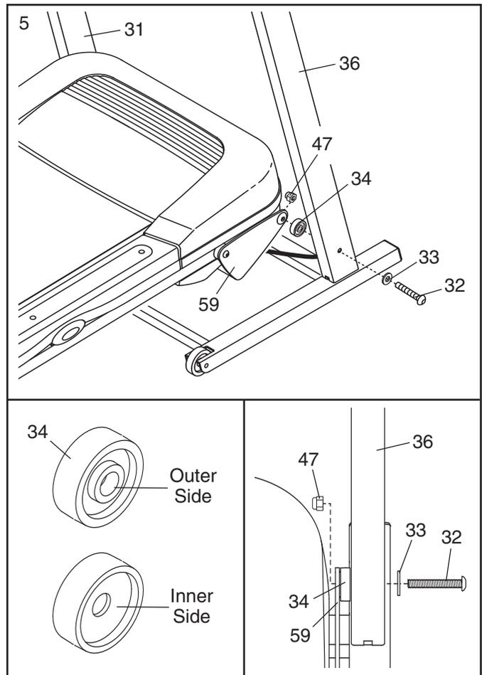
6. See the left inset drawing. Identify the outer side of the remaining Frame Spacer (34).
