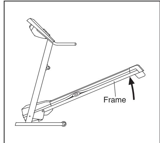
2. Move your right hand to the position shown and hold the treadmill firmly. Using your left hand, pull the latch knob to the left and hold it. Raise the frame until the hole in the isolator is aligned with the latch pin, and then slowly release the latch knob. **Make sure that the latch pin is fully inserted into the center of the isolator.**
