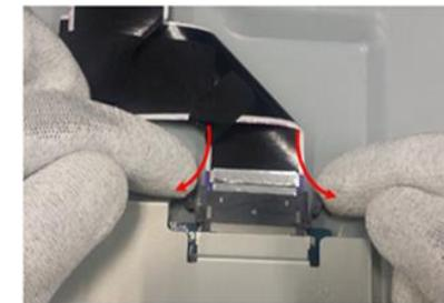
Do not bend the ear lock during FFC insertion. Rough handling will cause ear lock at connector broken as in picture below:
