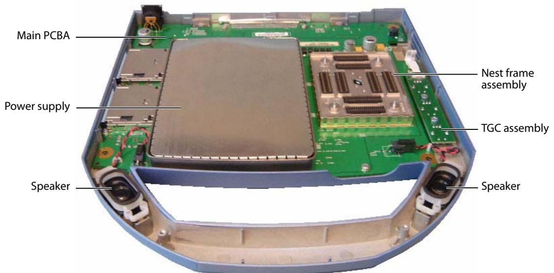
Figure 7.7 System Components
