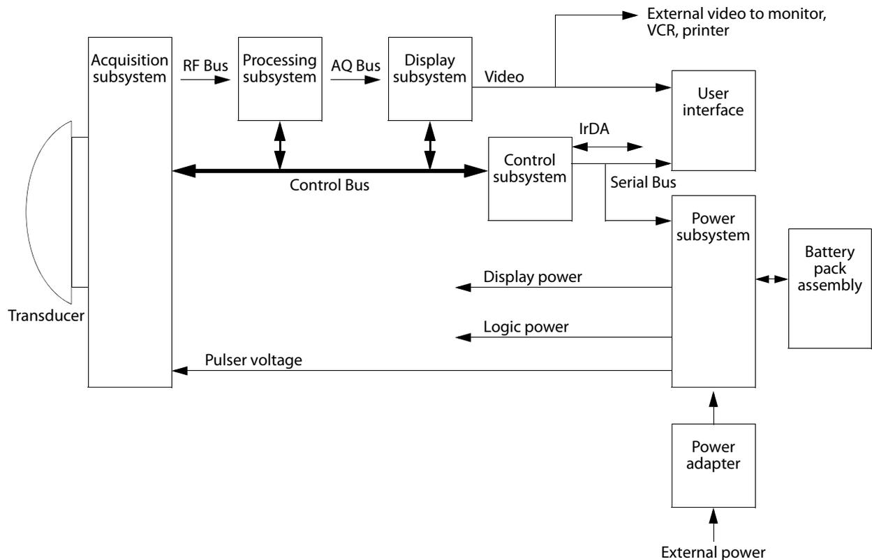
Figure 3.1 SonoSite High-Resolution Ultrasound System (MicroMaxx) Block Diagram
