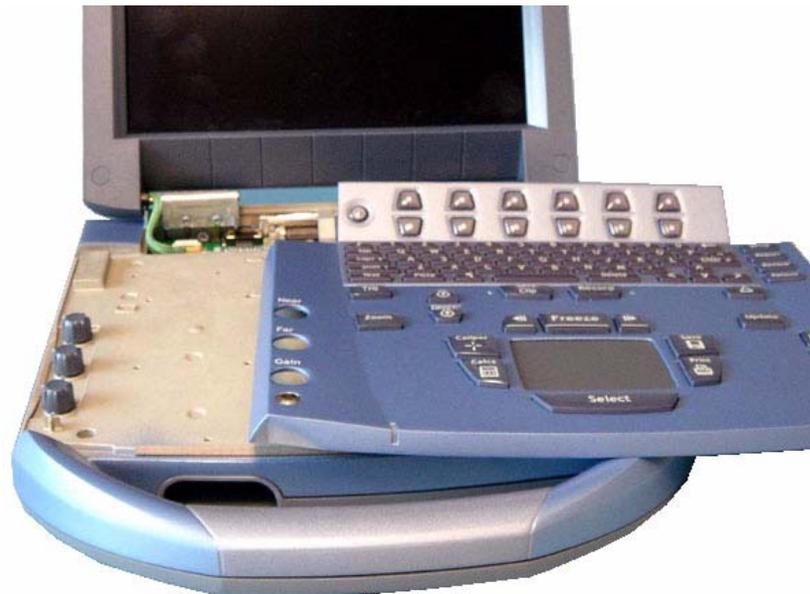
Figure 7.3 Control Panel Removal
