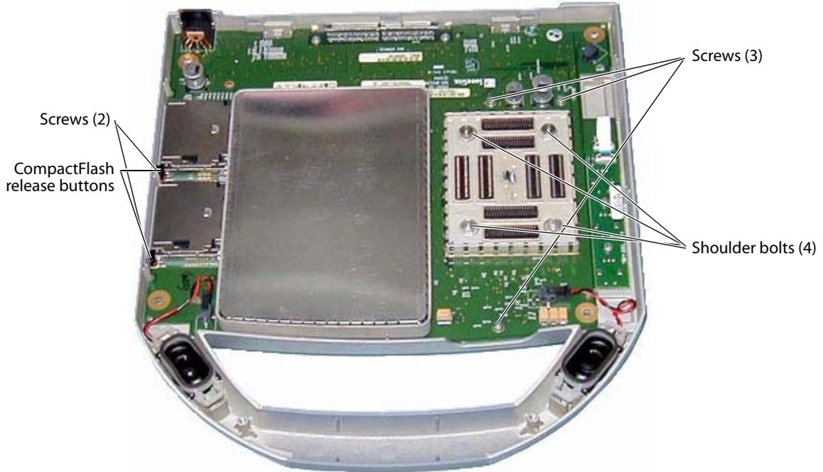
Figure 7.13 Main PCBA Screws
