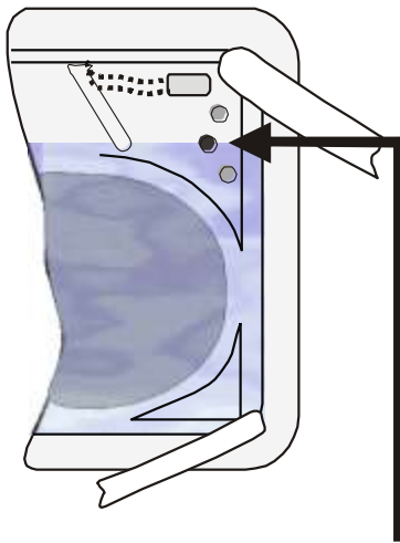
Proper water level is at 2nd level sensing pin
