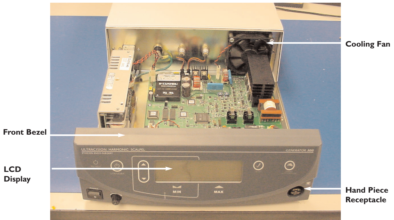
Fig. 12-1 Front Bezel Components and Cooling Fan
