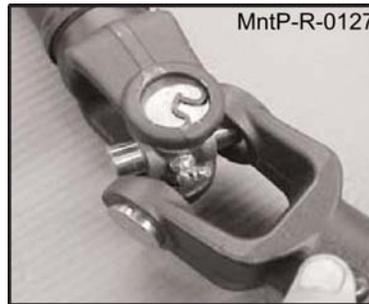
8. Grease Kit after assembly is completed.
