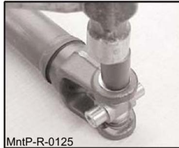
6. To loosen cross, strike yoke arm and check cross for free rotation
