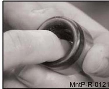
2. Insert cup and cross. Drive in with spacer.
