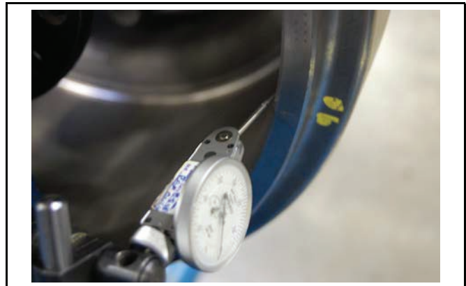
Measuring Runout with a Lever-Style Dial Indicator FIGURE 21
