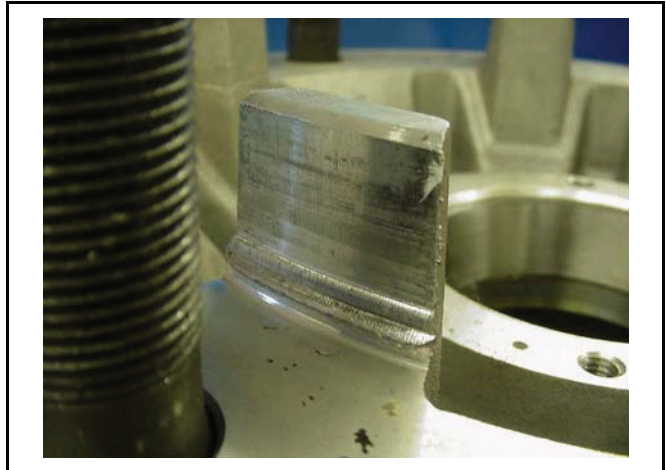
Damaged Pilot on Hub due to Drum Mismatch FIGURE 13
