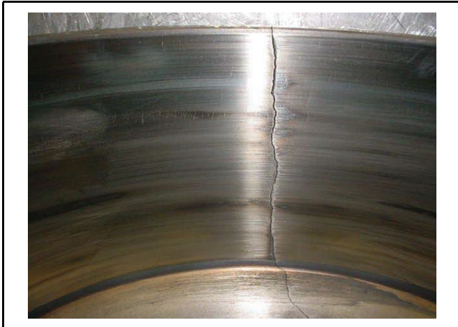
Cracked Drum Barrel FIGURE 11
