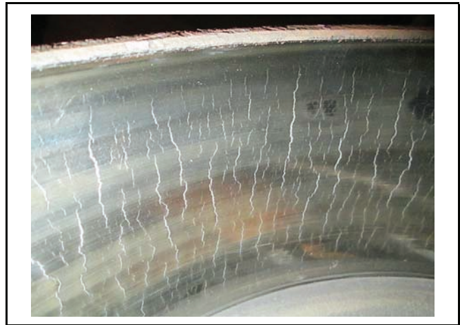
Heavy Heat Checks FIGURE 10
