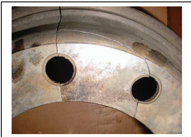
Cracked Mounting Flange FIGURE 12
