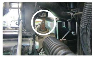
• Remove the steering gear assembly from the chassis by pulling it out to the right side of the vehicle then destroy the steering gear assembly.
