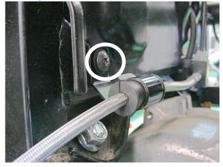
• Install the front shock absorbers and tighten the original bolts and new nuts from the repair kit to 57.5N·m (5.86 kgf-m, 42.4 ft-lb).
