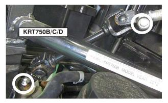
• Install and tighten the left-side brake hose mounting bolt.
