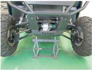
• Remove both front wheels and retain the nuts (and washers on the "C" model).
