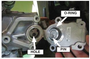
Install and tighten the shift actuator bolts in the sequence shown in the photo to 9.8 N·m (1.0 kgf-m, 87 in-lb).
