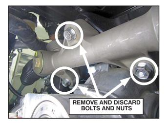
• Remove the steering gear assembly from the intermediate shaft.
