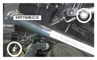
Install the new steering gear assembly bolts and nuts from the repair kit and tighten to 95.5 N·m (9.74 kgf-m, 70.4 ft-lb).
