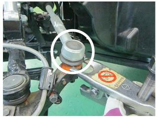
• Remove the front shock absorbers and retain the upper and lower mounting bolts. Discard the nuts.
