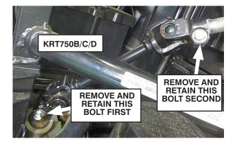
• Remove and retain three bolts to free the shift actuator.
