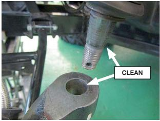
Install the left and right tie-rod end joints into the left and right steering knuckles and install the washers and nuts and tighten to 41.5 N⋅m (4.23 kgf-m, 30.6 ft-lb).
