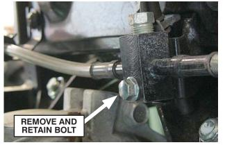
• Remove and retain the right-side brake hose clamp screw to free the brake hose.
