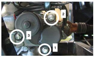
• Tighten the intermediate shaft clamp bolts to 21.5 N·m (2.19 kgf-m, 15.9 ft-lb).
