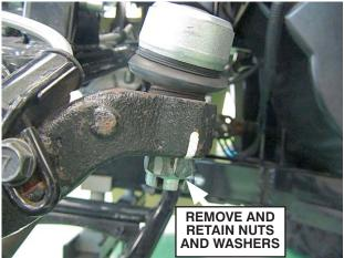
• Remove the tie-rod ends from the steering knuckles from both sides of the steering gear assembly using a suitable joint tool.
