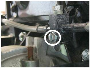
• Install and tighten the right-side brake hose clamp screw.
