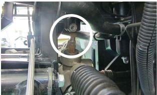
• Temporarily tighten the intermediate shaft clamp bolts.
