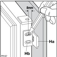
Remove the brackets and mark a distance of 8 mm from the outer edge of the door where the nail must be fitted (K).
