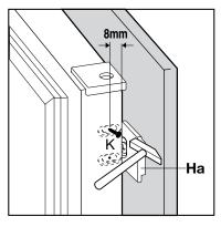
Place the small square on the guide again and fix it with the screws supplied.
