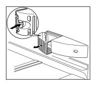
press on the rear hook and at the same time slide the cover in the direction indicated by the arrow. Unscrew the bulb and replace it with one of the same
