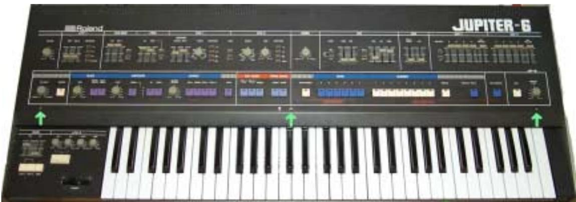
**Figure 2 – JP-6 front panel screw locations**
