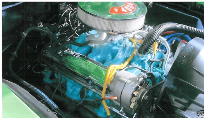
ENGINE REPAINTED (WRONG COLOR) FIREWALL & FAN SHROUD REPAINTED. ALTERNATOR HOOKED UP WRONG
