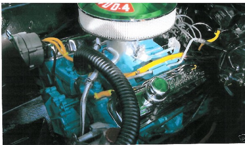
INTAKE IS STILL 2 BARREL w/ 67 C. CARB & CLEANER w/ 400 TAG NOTICE RED PS CAP NOT HOOKED UP. NO DYNAMAT NOW.
