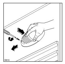
Remove the screw from the light cover and then pull it outward toward the middle of the cabinet. Unscrew the bulb and replace it with a new 15 watt bulb (available from your nearest Service Force Centre).
