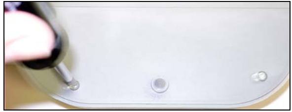
Figure 3-4. Removing screws that secure the PCB Cover.
