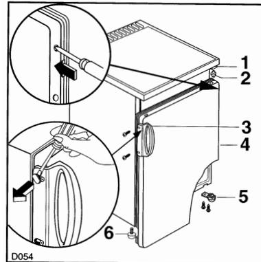
**When positioning the bottom hinge blade on the reverse side, the securing screws will require a degree of exertion when fitting. It is therefore advisable to lubricate the screw tips before starting this operation.**
