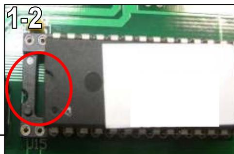
3. Line the legs of the chip with the slots in the socket and push the chip
