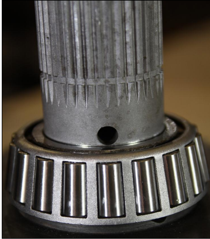
Figure 47-tapered roller installed on shaft while in main case
