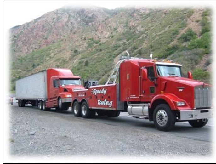
Figure 2-flat towing should be avoided when possible
