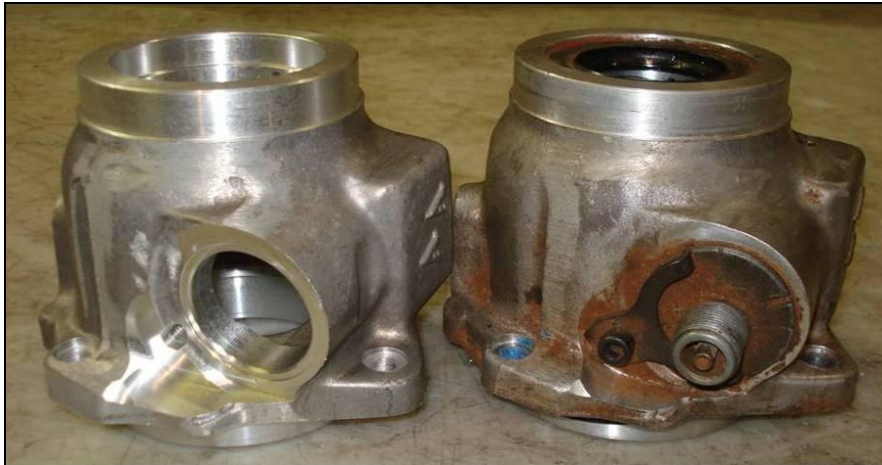
Figure 5-shows correctly cleaned housing on left and dirty housing on right
