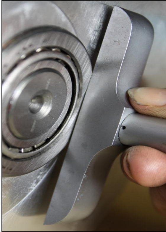
Figure 42-measurement of bearing race height
