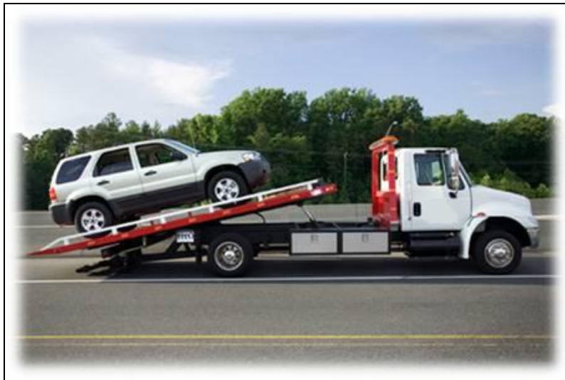
Figure 3-raised towing is the preferred method
