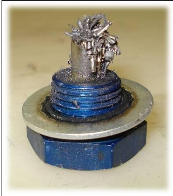
Figure 8-excessive debris indicates problem
