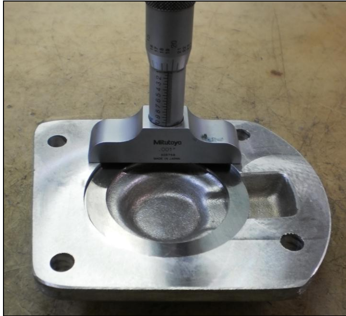
Figure 44-depth measured with shims installed
