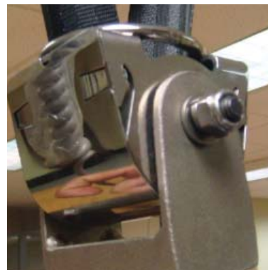
5.5 Remove securing nuts and pin to remove carry bar
