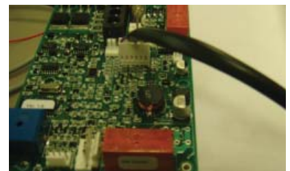
7.9 Hand Control connector (Connector #3 - 6 pins)
