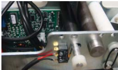
7.17 Reinstall the upper limit switch roller and O-ring
