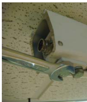
1.6 Loosen end stop bolts
