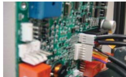
7.11 Limit Switches (Connector #5 - 3 pins)
