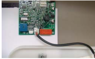
7.8 Traversing Motor (Connector #2 - 4 pins)
