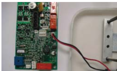
7.10 Hour Meter (Connector #4 - 2 pins)
