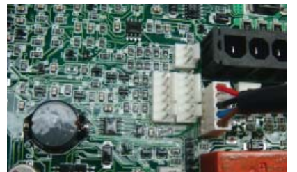
7.13 Main Housing LEDs (Connector #7 - 5 pins)
