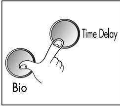
Check on the spinning, is the frequency of the water level 248 or more. The frequency can be checked by pressing the **Bio** and **Time Delay** buttons at the same time on the program.
