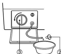
Unplug the drain plug (②), then the water flows out. At this time use a vessel to prevent water flowing on the floor. If the water does not flow any more, turn the pump filter (③) open to the left.
