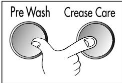
When pressing **Pre Wash**, **Crease Care**, and **POWER** buttons at the same time after power off, press the **START/PAUSE** button 2 times, is the drum low speed spin?
