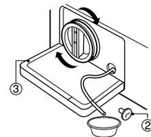
Take out any foreign material from the pump filter (③). After cleaning, turn the pump filter (③) clockwise and insert the drain plug (②) to the original place. Close the lower cover cap.
