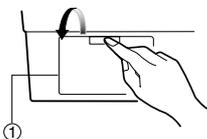
Open the lower cover cap (①) by using a finger. Turn the drain plug (②) to pull out the hose.
