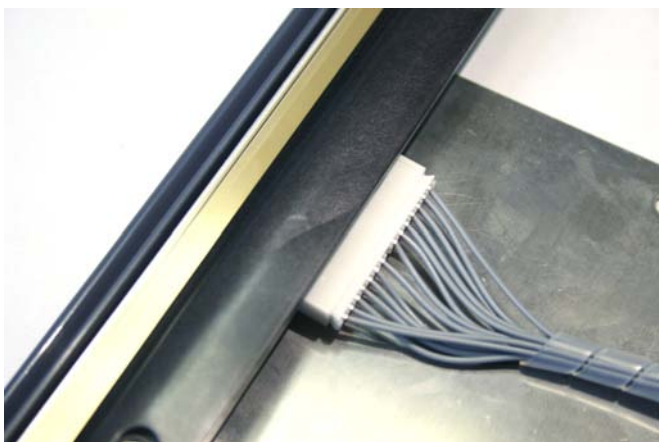
3. Attach the Printer Cable
