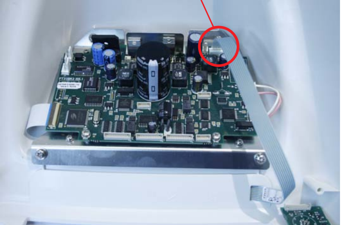
13. Connect the Control Panel cable
