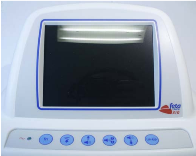
12. Attach the LCD label to the enclosure
