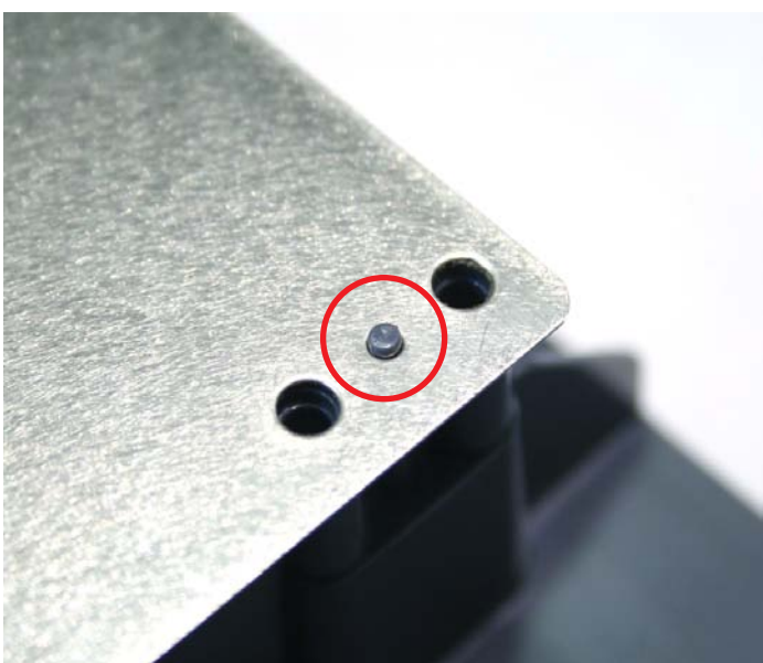
4. Place the springplate over the mounting posts
