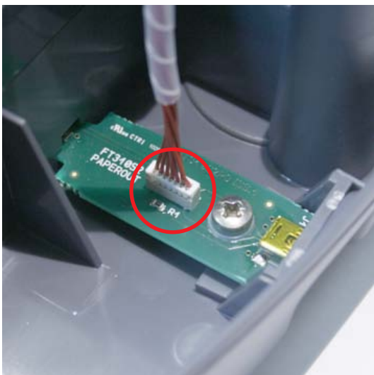
1. Connect the Paper Out Cable
