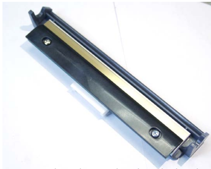
2. Place the Printhead on the bracket
