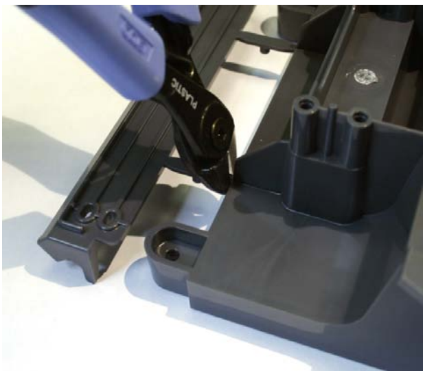
1. Cut away the Printhead bracket
