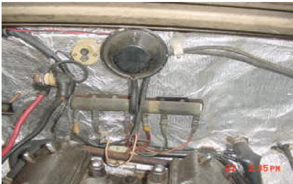
A 420 resistor set-up
