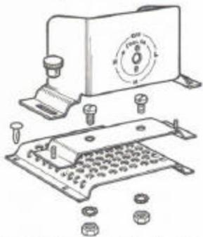
Fig. 21. Attachment of control unit panel.
