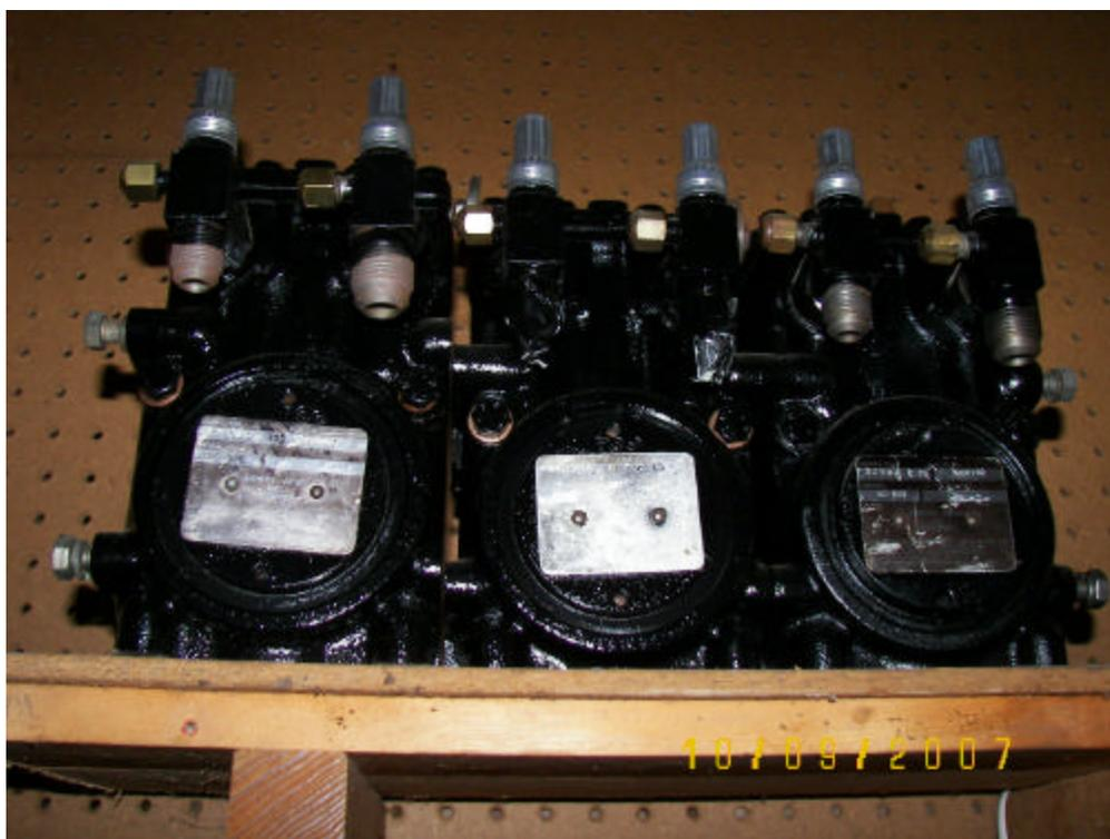
This photo also serves to show proper valve finish on the Tecumseh HG500 compressor – brass service caps and aluminum valve stem dust covers – not plastic. Also note the valve bodies are steel and not aluminum, as were the later replacements.
