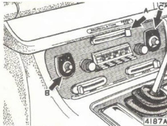
**'Delanair' Air Conditioning System As Fitted To 2.8 Litre and 4.2 Litre Jaguar XJ.6.**
