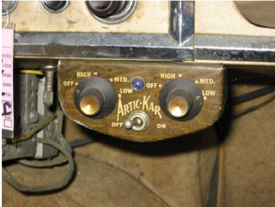
A typical set of control switches. There are two fan speed switches and a compressor on off switch with a blue ON lamp. Note the period LOGO and the wood grain lithograph is unique to this author.
