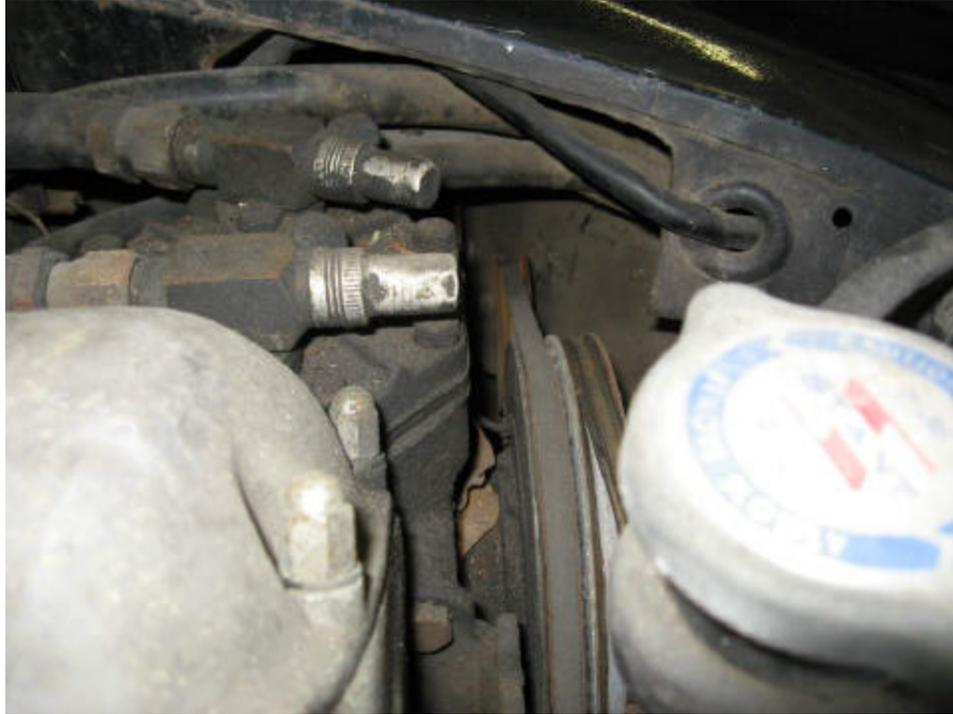
Of interest in this picture the inner wing has been cut to allow for the compressor. A box cover was fabricated for the wheel side to cover the opening and protect the compressor and generator (under the compressor).
