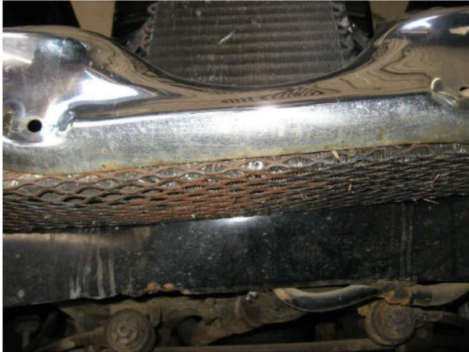
The under bumper and secondary condenser. Note the rock guard.
