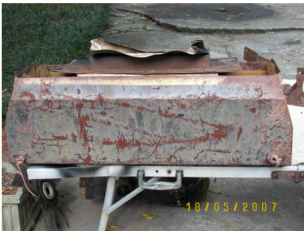
The evaporator case removed from a MK VII M. It has an unusual coffin shape – the remnants of the Jaguar decal were there, but not visible in the photo
