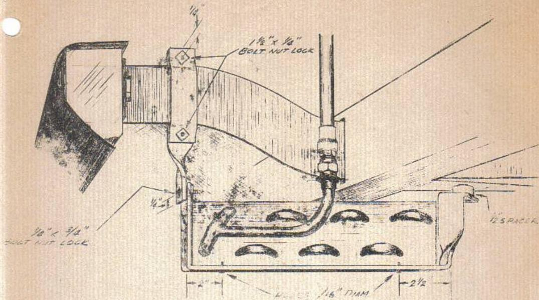
The mounting, as depicted above, should position the condenser at approximately a 15 degree angle with the rear of the condenser lower. The clamp which positions around the bumper arm can be left loose, i.e. the bolts and nuts finger tight, so that it can slide on the arm for ease of installation. The brackets fix to the condenser flanges by two each #8 x 1/2 SMS.
