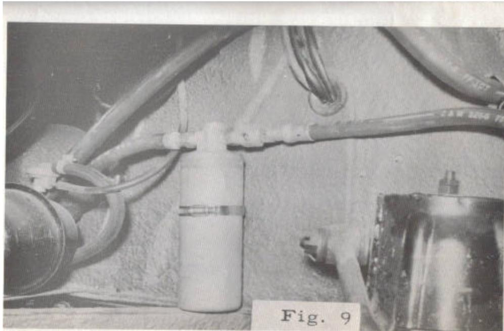
Receiver drier mounted in the wheel well of the S-type / MK2
