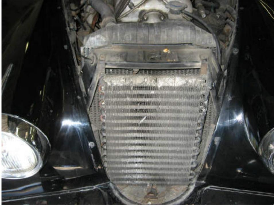
The main condenser mounted in front of the radiator.
