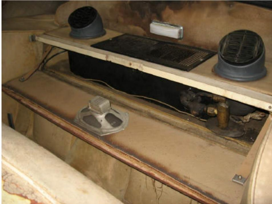
A more complete picture noting the rear compartment has been modified for the AC yet has been covered with the proper materials. This was typical in the period.
