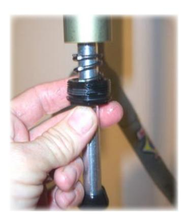
49) Re-install the Wind Down Compression Rod and tighten the end cap.
