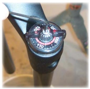
42) Use a 2mm Allen wrench to loosen the adjuster knob set screw.
