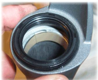
18) Start the seal into the lower leg and use your thumbs to press it down evenly until flush with the top edge of the lower leg.
