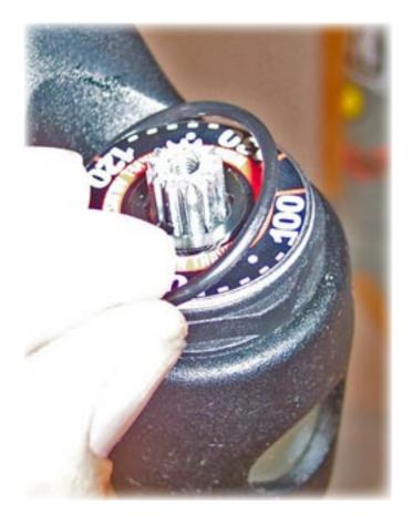
44) Remove the O-ring from around the travel scale.
