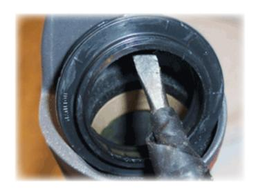
10) Apply downward pressure on the screwdriver handle until the wiper/seal "pops" up and out.
