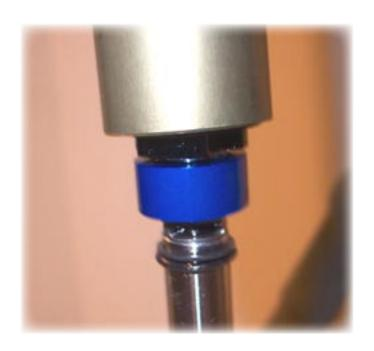
33) CAREFULLY insert the SPV/rebound damper assembly into the stanchion tube.
