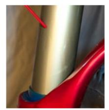
Drizzle some Stanchion Lube<sup>TM</sup> onto the clean stanchion tubes and allow it so settle on the tops of the wipers.
