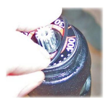
53) Replace the O-ring around the travel scale.
