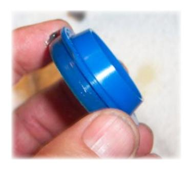
20) This is the Enduro Wiper. Apply a thin coating of grease to the insertion area of the wiper.
