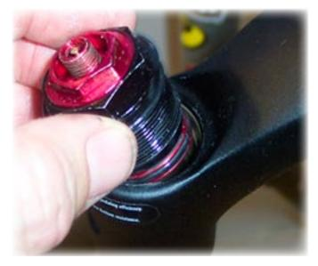
39) Start the top cap into the top of the leg by hand.
