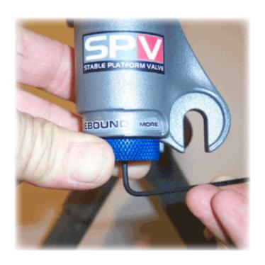
3) Adjust the rebound knob mid-way and use the 2mm Allen wrench to remove the retaining screw.
