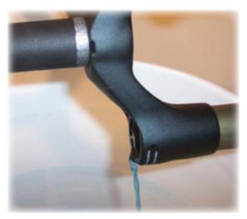
26) Pour the damping oil out of the chamber.
