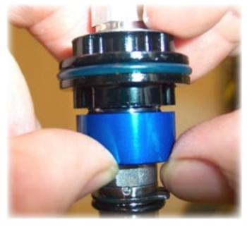
The valve should spring back to the open position when you release it.
