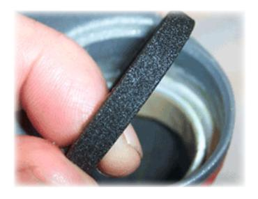
11) Remove the "foam ring" from the seal insertion area.
