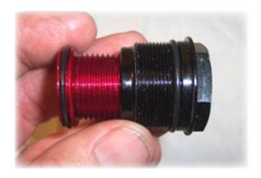
This is what the top cap assembly looks like with the adjuster hex wound all the way IN. This is how volume is reduced in the air chamber.
