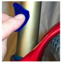
Compress the fork a few times. Using a soft cloth, work the excess Stanchion Lube<sup>TM</sup> into the upper legs. Repeat until no residue remains.
