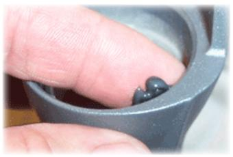
17) Use some Super-Slick Grease®, Prep-M® or other supsension compatible grease to lubricate the outside edge of the inner oil seal and the seal-insertion area of the lowers.
