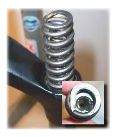
Slide the main spring down into the fork leg until it contacts the top of the Compression Rod assembly. Slowly rotate the spring until the the "D"-shaped spring end aligns with the "D"-shaped top of the Compression Rod assembly (you will feel the spring drop into place).
