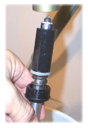
48) Remove the Travel Wind Down Compression Rod assembly from the stanchion tube.
