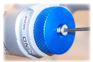
62) Insert and tighten the Rebound Knob set screw, using a 2mm Allen wrench.
