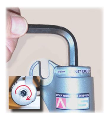
4) Invert the fork and use the 8mm Allen wrench to wind the damper rod CLOCKWISE into the lower leg.
