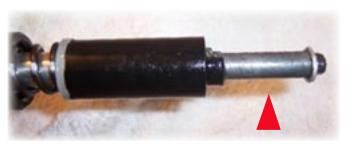
When the fork is assemble and you adjust the Travel Wind Down Knob, the "D"shaped main spring end drives the black spacer up and down the Wind Down Compression Rod.
