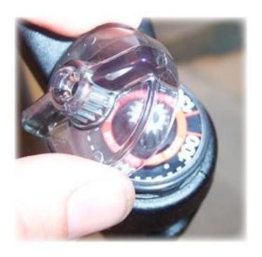
43) Lift the adjuster knob straight up and off of the top cap assembly.
