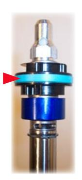
29) Verify a gap of approximately 1mm between the blue SPV valve and the black piston.
