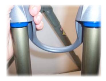
56) Start the lowers over the rods and down to the stanchion tubes. *Be sure the reverse arch is facing the right way*.
