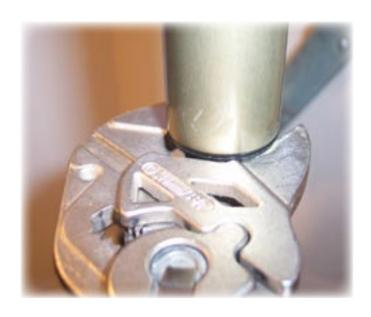
34) Use good-quality adjustable flat jawed pliers or a wrench to tighten the damper end cap.
