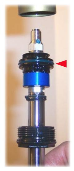
28) Remove the SPV/rebound assembly from the stanchion.
