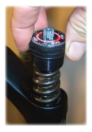
46) Remove the top cap and coil spring.
