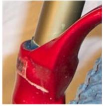
For longevity, it is important to keep the stanchion tubes and top edges of the wipers clean. (Note the dust ring on top of the wiper.)
