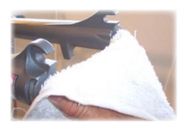
59) Cover the lower casting holes with a clean towel to prevent oil from being ejected and push the lower assembly all the way onto the stanchions.
