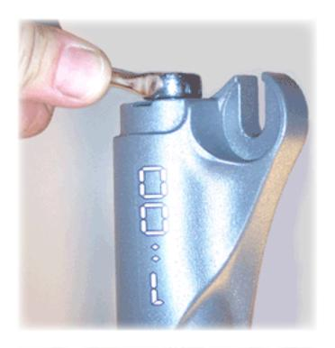
5) On the spring side (rider's left), use a 7/16" wrench to remove the bottom fixing bolt.
