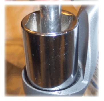
19) Use a large inverted socket and extention to carefully seat the inner oil seals in each leg.
