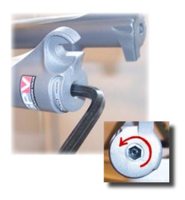
60) Use the 8mm Allen wrench to wind the SPV/Rebound damper rod back into the lower leg casting.
