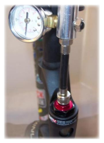
41) Pressurized the SPV air chamber to about 40 PSI.
