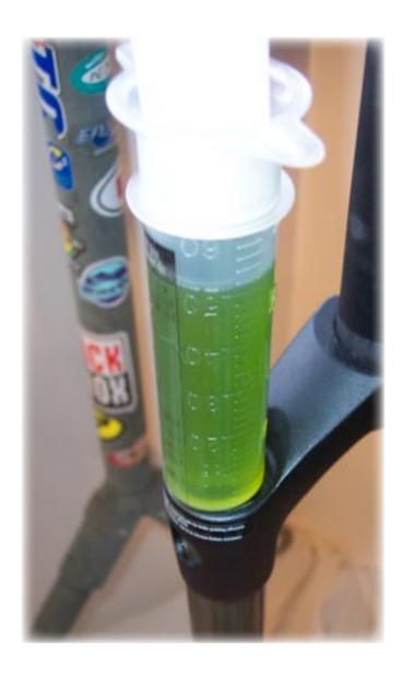
36) Repeat step 35 so that the total suspension fluid added is about 120cc.
