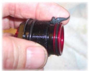
38) Lightly lubricate the threads and both O-rings on the SPV top cap.
