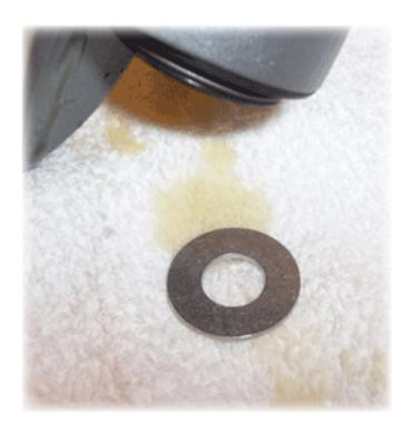
7) After draining the oil, invert the lower assembly to remove the bottom washers.
