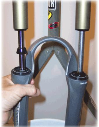
6) OVER A BUCKET OR OIL PAN, turn the fork back over, drain the semi-bath oil out of the lower assembly, and pull the lower assembly off of the stanchions.
