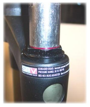
24) Use a 5/8" or 16mm socket on the red adjuster hex back out the entire SPV top cap.
