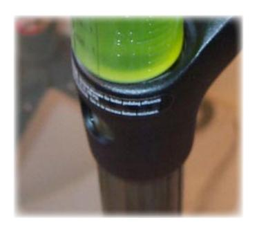
Insert the syringe and tubing into the fork leg until the syringe body is resting against the crown. Remove it and look for fluid on the end of the tubing. If the tubing did not contact fluid, add fluid until it is higher than the end of the tube. Re-insert the syringe with the plunger fully compressed into the syringe body. Holding the syringe against the crown, pull the plunger up, removing the excess oil until only air is being pulled into the syringe. You are now at a level of 84mm.
