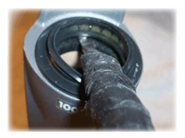
9) Insert a flat-bladed screw-driver under the back end of the seal/wiper.
