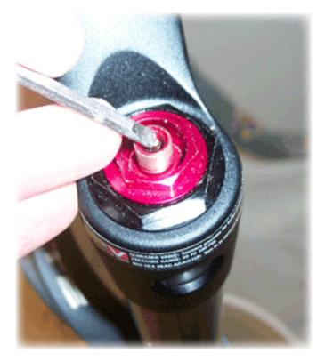
2) Remove the Schraeder valve cap from the SPV side and carefully relieve the air pressure.
