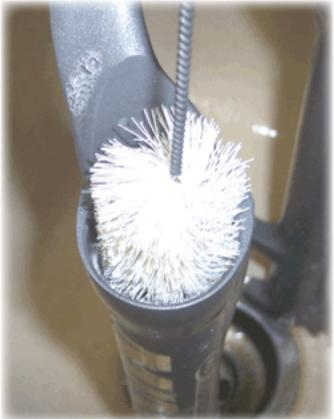
13) Chase the degreaser with a mixture of hot water and dish soap and a little brushing, if needed. RINSE well with hot water.
