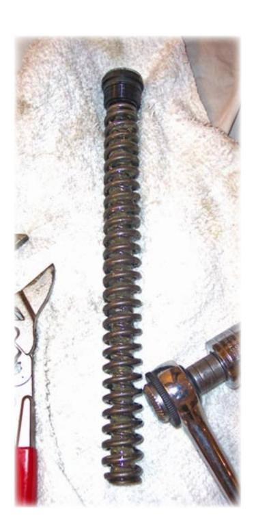
This is the stock coil spring with the top cap still in the end of it. Notice the smaller diameter spring interwined in the center of the main spring. This is called the "Booster Spring." The stock configuration is considered "Medium."
