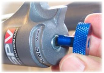
61) Carefully line up the Rebound Adjuster Knob and push it up into the bottom of the damper rod.
