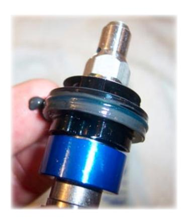
31) Apply a light coating of a suspension-friendly grease such as Super-Slick Grease® or Prep-M® on the O-ring or Teflon® seal (depending on whether you are using the SPV or the SPV Evolve cartridge).
