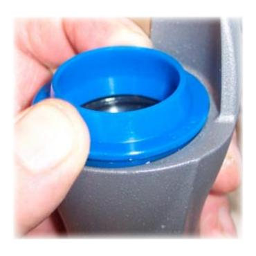
21) Start the wiper into the insertion area of the lower leg. It should be easy to start, as the leading edge is slightly tapered.
