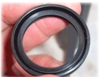
15) This is the BOTTOM of the inner oil seal. See the deep groove? IT FACES DOWN.
