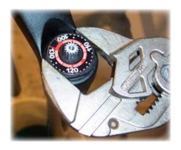
45) Loosen the Travel Wind Down top cap using good-quality adjustable flat jawed pliers or a wrench.
