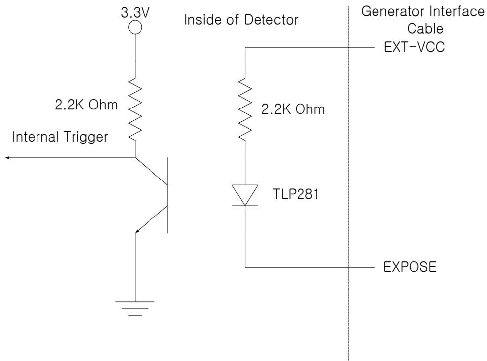
Note : To activate trigger function, the current through LED of TLP281 should be in the range of 5.5mA to 16mA, so the voltage between VCC-EXT and Expose pin should be in the range of 12V to 36V .
