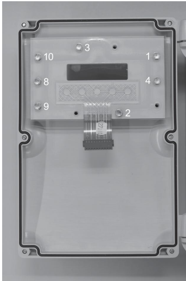
Figure 2-3 Keypad Assembly (P/N A5E03056923)
