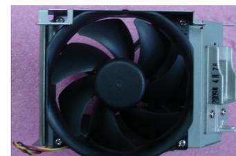
2. Unscrew 4 screws (as blue circle) to separate System Fan and System Fan Shielding.
