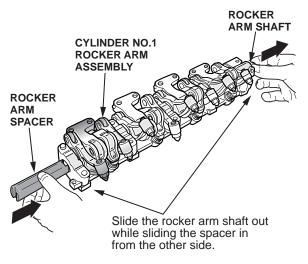
While pushing in the rocker arm spacer, slide the rocker arm shaft out of the cylinder No. 1 rocker arm assembly. Make sure to keep the holder grooves vertical.
