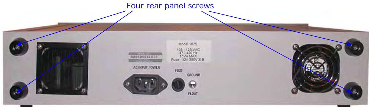
Figure 3.2 Location of four rear panel screws
