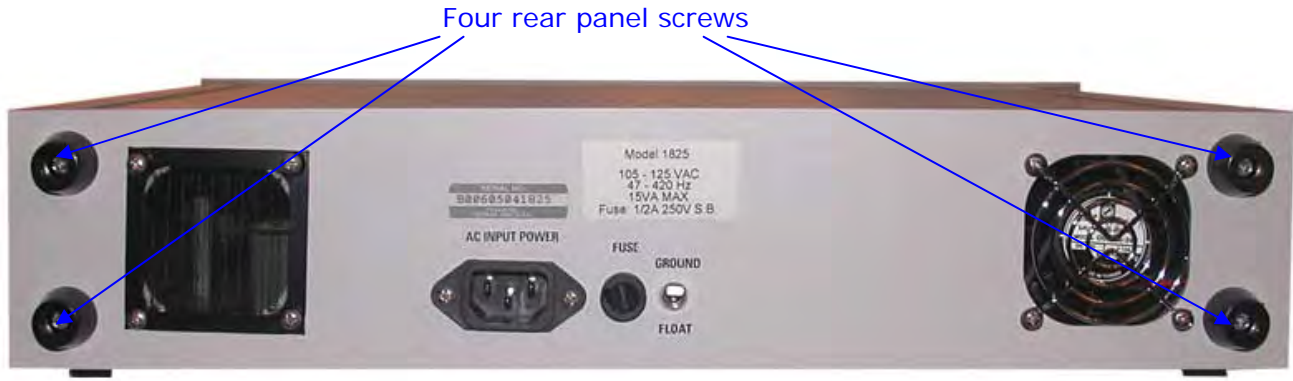
Figure 4.2 Location of four rear panel screws
