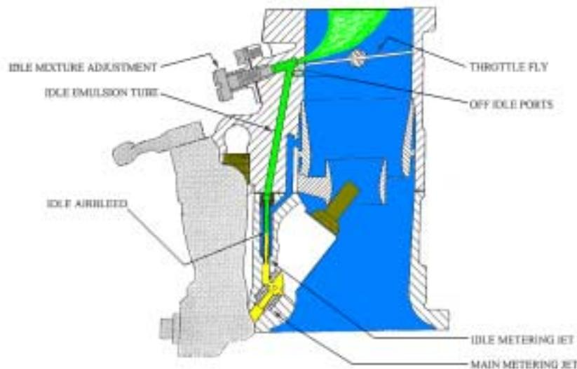
FIGURE 1. TYPICAL IDLING SYSTEM IN A FLOAT CARBURETOR.
