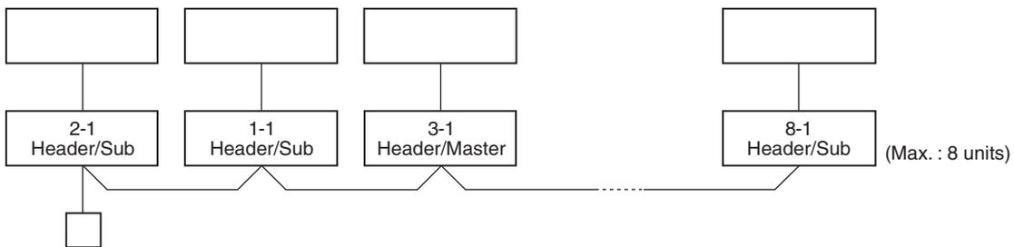
**Only turning on source power supply (Automatic completion)**
