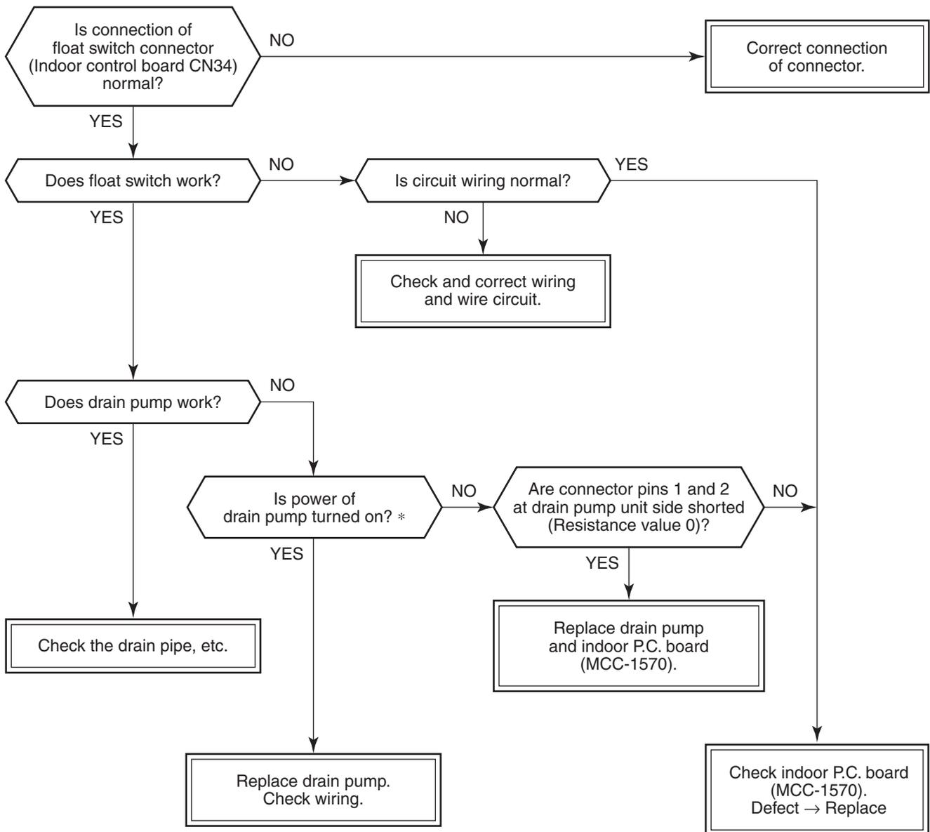
\* Check that voltage of 1-2 pin of CN504 on the indoor P.C. board is +12V. (1 pin is plus (+).)
