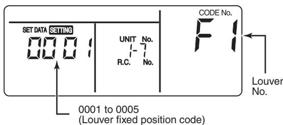
\* F1 displayed at the CODE No. on the remote controller means that the 01 louver was selected as shown in the figure.
