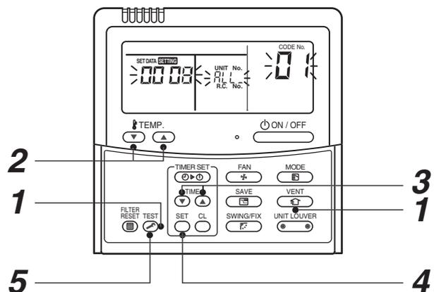
**How to confirm the central control address (New function for AMT32E remote controller)**
