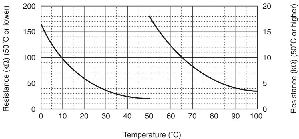
\* As TH sensor (Outdoor unit heat sink temp. sensor) is incorporated in the outdoor control P.C. board, the resistance value cannot be measured.
