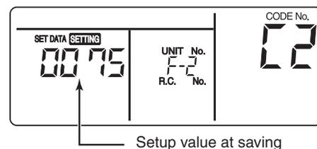
**4** Push **SET** and then push **TEST** to finish the setup.
