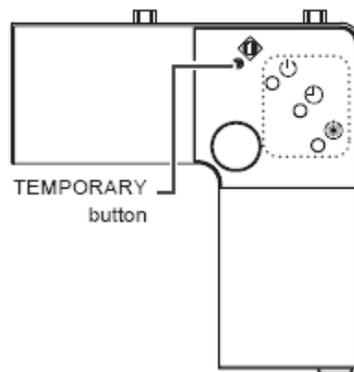
**8-1-2. Forced Defrost Setup of Remote Controller (For wired remote controller only)****(Preparation in advance)**
