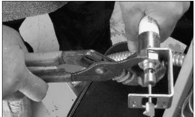
Tighten the nut on the Dawson tube assembly.
