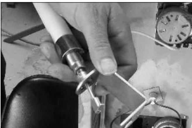
Installing the bracket to the new tube assembly (Dawson tubes).
