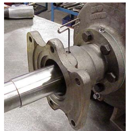
Figure 20, Setting the driving ring
