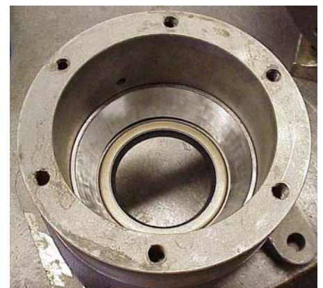
Figure 13, Inner bearing race installed
