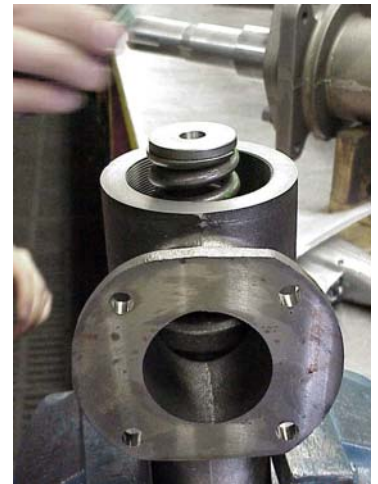
Figure 28, Spring and retainer installed
