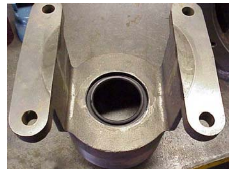
Figure 12, Inner lip seal orientation
