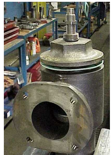
Figure 29, End cap, adjusting screw & locknut
