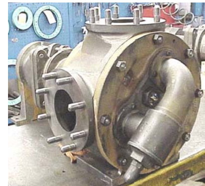
Figure 2, Standard head and relief valve orientation.
