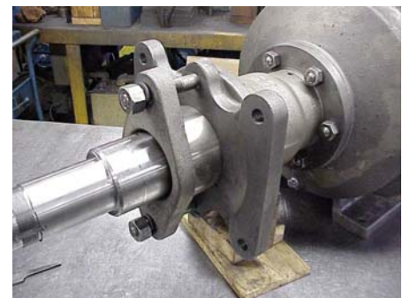
Figure 11, Packing gland installed
