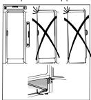
there is good air circulation around the cabinet and that the air channels below and behind the cabinet are not blocked. The ventilation space above the cabinet must be at least 4 cm.
