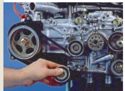
Removing Idler Pulleys
