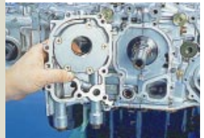
Installing Oil Pump
