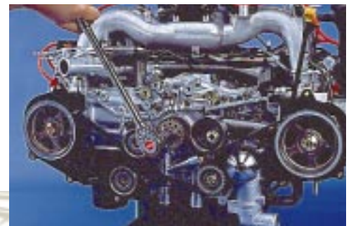
Checking Cam Belt Alignment
