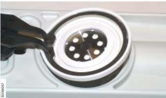
To remove the valve membrane from the cassette:
