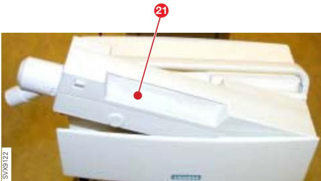
The expiratory cassette (21) is a complete unit and must not be disassembled. It contains the following parts:
