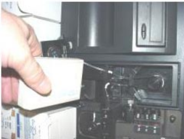
Figure 5.2 Inserting the Optical Calibration Tool into the Cuvette Slide Housing
