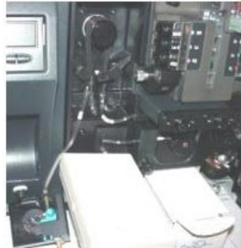
Figure 5.2 Inserting the Optical Calibration Tool into the Cuvette Slide Housing
