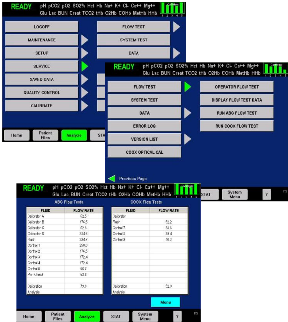
Figure 4.11 ABG and COOX Flow Tests Data Screen
