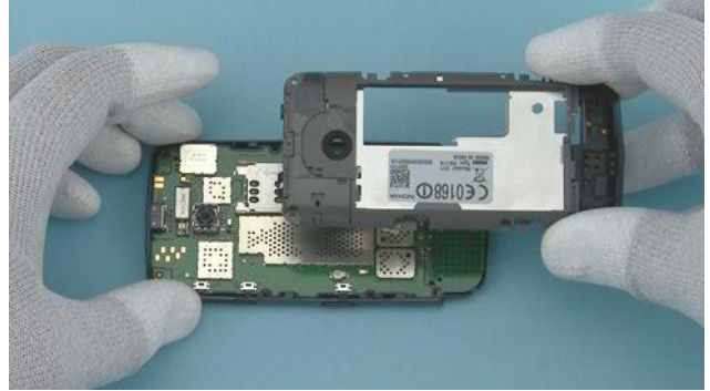
14) Remove the B-COVER and the ANTENNA MODULE ASSEMBLY.
