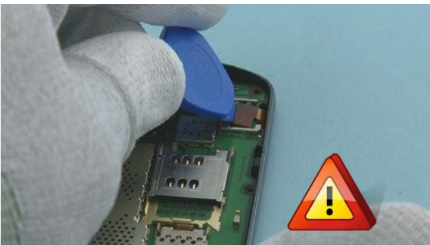
21) Open the DISPLAY CONNECTOR with the SRT-6. Be careful not to damage the connector.
