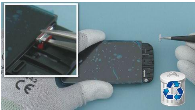
9) Remove the END KEY with tweezers. Do not use it again.
