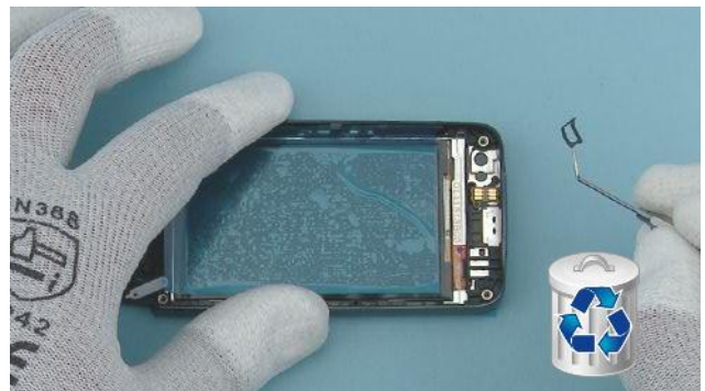
36) Remove also the EARPIECE residues from the A-COVER.
