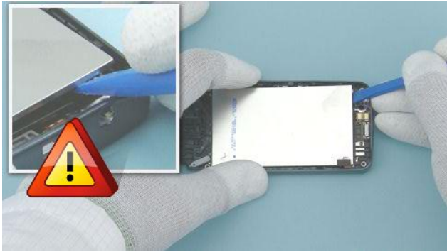
31) Lever up carefully the DISPLAY with the SS-93.
