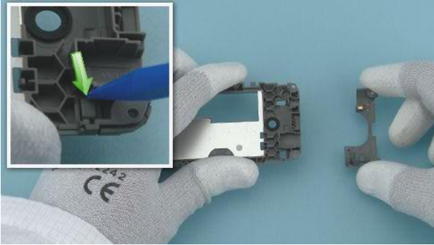
19) Release also the second clip with the sharp end of the SS-93. The B-COVER and the BT ANTENNA MODULE can now be separated.
