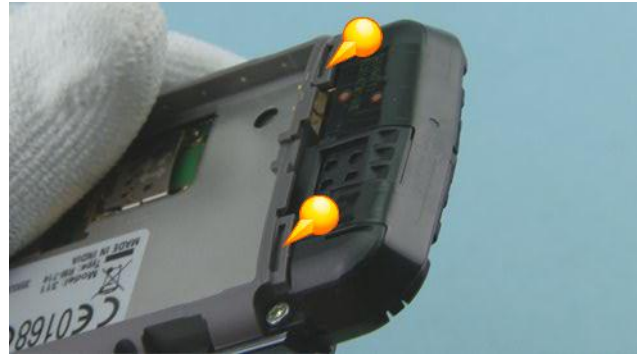
8) Check that the A-COVER hooks did not get damaged during disassembling of the ANTENNA COVER.
