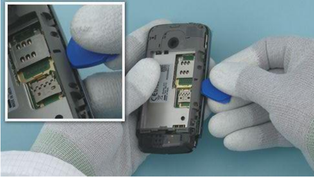
13) Use the SRT-6 to release the B-COVER.
