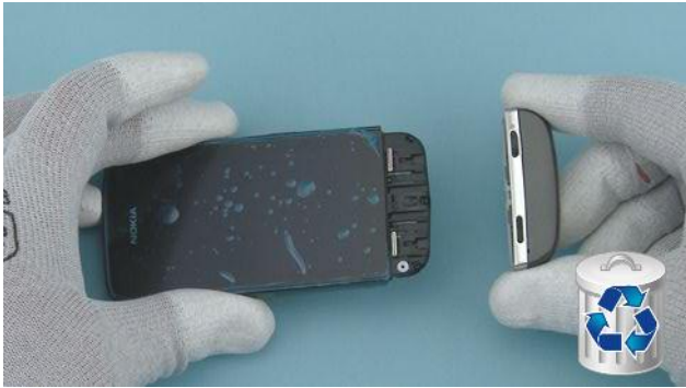
7) Pull out and remove the ANTENNA COVER. The ANTENNA COVER is not reusable. Discard it.
