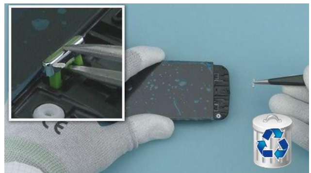
10) Remove the SEND KEY with tweezers. Do not use it again.
