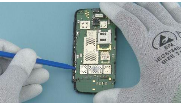
23) Release also the other side of the ENGINE BOARD with the SS-93.
