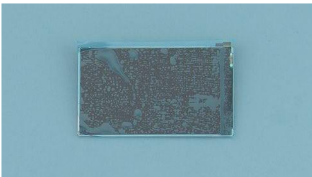
33) Protect the DISPLAY with protective film.
