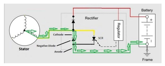
The electrons will flow from the stator to the negative battery terminal during the part of the AC wave that is at least -.7 volts more negative than the zero voltage the anode is tied to at the negative battery terminal.
