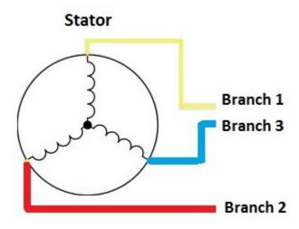
Each branch outputs an AC voltage, but they are not all in sync with each other. Each branch is 120 degrees *out of phase*. The graph below shows each phase of the three branches.
