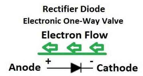
Electrons will flow from Cathode to Anode when the Anode voltage is .7 volts higher than the Cathode voltage.
