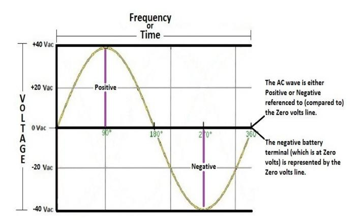
At the beginning of the wave we are at zero volts. As you follow the wave it climbs in a positive direction until it reaches it's peak and begins to fall back to zero. Any point above the zero volts line is said to be positive.
