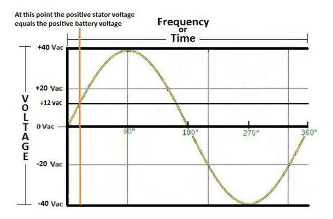
From this point on the yellow branch of the stator will be *more positive* than the +12 volts at the positive battery terminal. Once the stator voltage at the anode of the positive diode hits +12.7 volts the positive rectifier diode will "turn on" and electrons will start flowing from the positive battery terminal, through the positive diode, and into the yellow branch of the stator.
