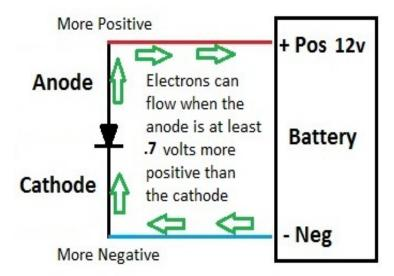
In this circuit the anode is now more positive than the cathode by +12 volts. The diode is now "on" and the electrons can flow freely. Let's take another look at the rectifier diodes and the battery from the charging system diagram.
