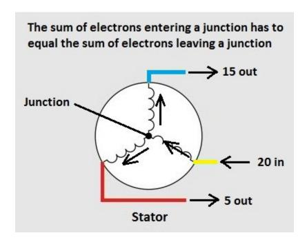
When we used the simple charging circuit diagram to show you how the stator, diodes, and battery work together we only used the yellow branch of the stator. We only showed the electrons flowing in and out of the yellow stator branch. From the above diagram you can now see that in order for the electrons to flow into the yellow stator branch they must also be able to flow out of either the red branch, the blue branch, or both.
