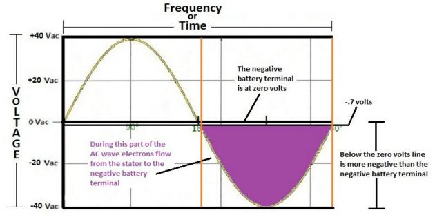
So what happens during the part of the AC wave that passes in the area below +12.7 volts and above -.7 volts on the graph? Nothing. No electrons are flowing in the yellow stator branch during this time because neither the positive or negative diode is turned on.
