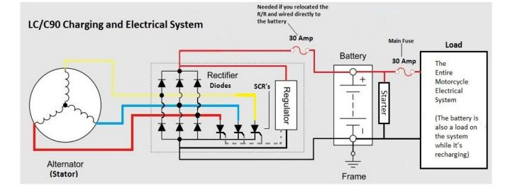
As you can see the cathodes are towards the positive battery terminal and the anodes are towards the negative battery terminal. The electrons cannot flow from the negative battery terminal to the positive battery terminal because the diodes are not "turned on" when oriented this way in the circuit.
