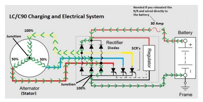
A few things to point out in the above diagram. We will use percentage of electrons as we traverse around the circuit. Also, notice there are two junctions marked. One is the junction in the stator. The other one is the junction at the bottom of the negative diodes.
