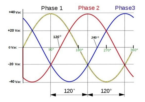
You will notice at the zero volts line the yellow branch is the first to start its upward swing. At 90 degrees it reaches it's peak. At 120 degrees of the yellow branches wave take a look at the zero volts line. You will see that the red branch is now starting its upward swing. 120 degrees after the red branch starts its upward swing (240 degrees after the yellow branch) the blue branch now starts its upward swing. This process continues over and over. The three phase system is very efficient.
