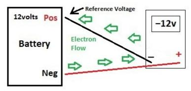
If you put the positive probe on the negative battery terminal, and the negative probe on the positive battery terminal, it will also read 12 volts...but the meter will display a minus sign by the number (-12).
