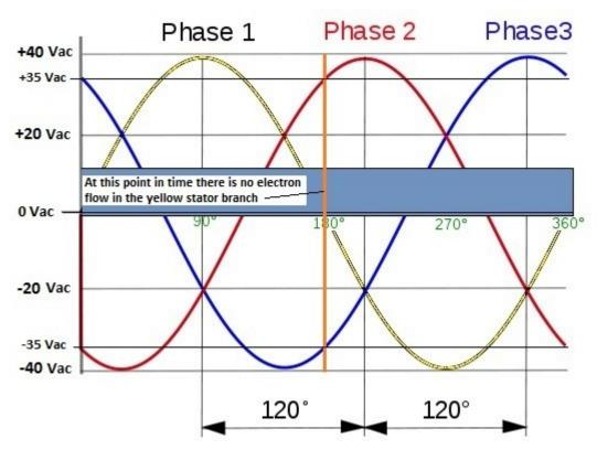
As you can see on the chart the yellow branch has no electron flow at all because it's passing through the region where neither of the diodes connected to it are turned on. All the electrons are entering the stator through the positive red branch diode and leaving the stator through the negative blue branch diode.
