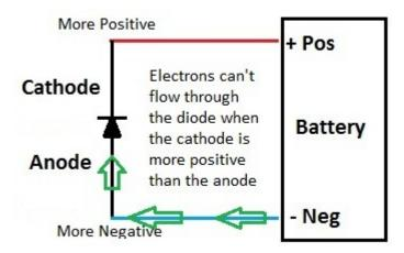
In the circuit above the electrons cannot flow from the negative battery terminal to the positive battery terminal because the diode is "off". It is off because the the cathode is more positive than the anode. Let's turn the diode around and look at it again.
