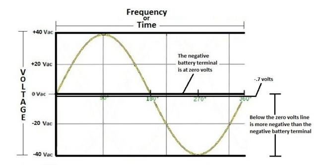
Once the stator voltage is -.7 volts the diode turns on and electrons flow from the stator to the negative battery terminal.
