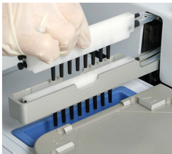
Figure 3–12. Fitting the 2 x 8 wash heads next to each other onto the wash arm
