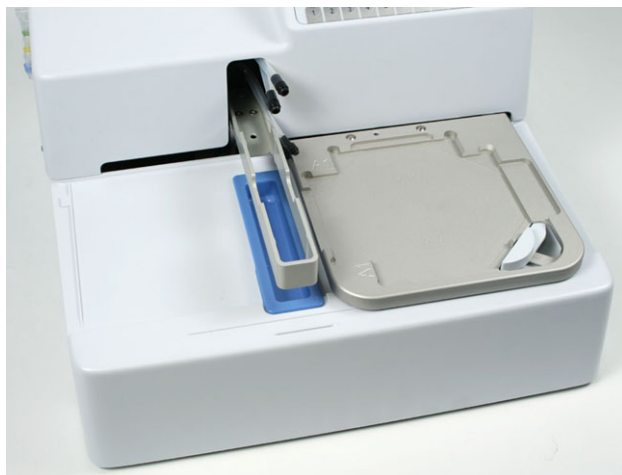
Figure 9-27. Aligning the plate carrier and wash head arm
