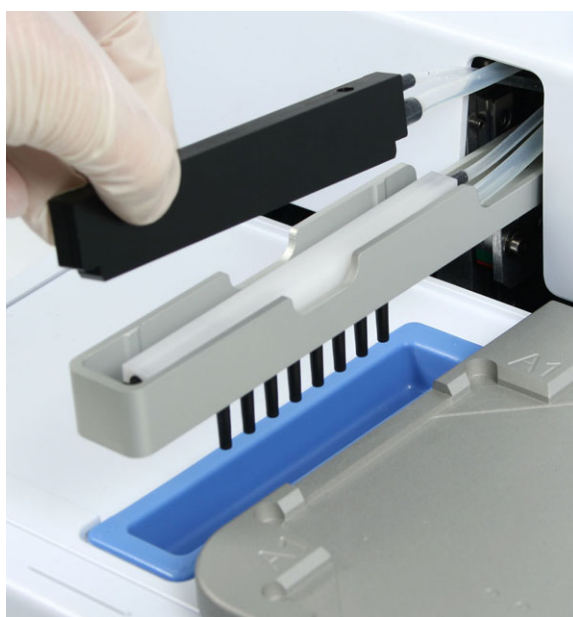
Figure 3–14. Fitting the blank wash head onto the left of the wash arm
