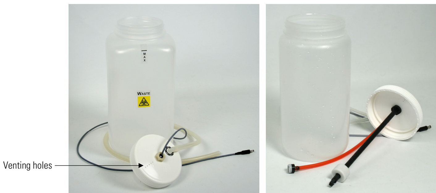
Figure 3–15. Waste and liquid containers with liquid level detection sensors
