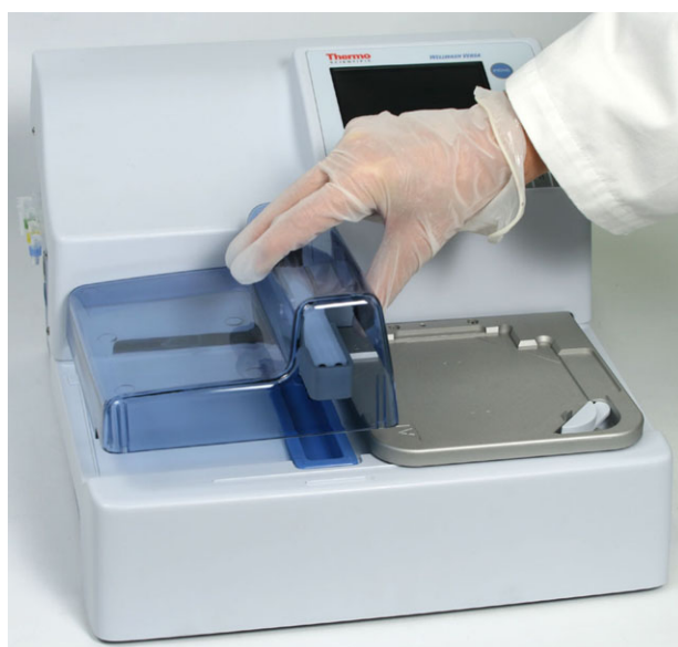
Figure 3–20. Magnetic mounting of the aerosol cover
