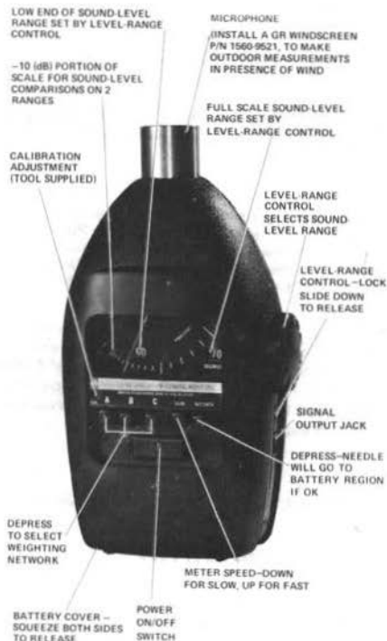
Figure 1-1. Sound-Level Meter Controls and Indicators.
