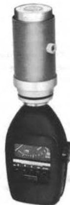
Figure 5-2. Type 1562 Calibrator mounted over SLM Microphone.
