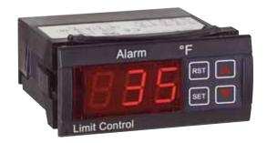
The Series TSF Thermocouple FM Approved Limit Control provides audible alarm status along with a robust 15 amp relay output. Unit allows the user to easily select automatic or manual reset along with 10 other parameters. The TSF series has a built in reset button on the front panel or can accept an external reset.
