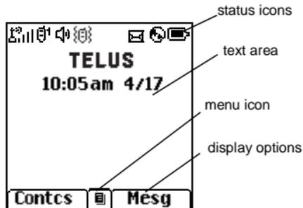
The screen shown above is the idle screen. The idle screen appears when your handset is on, but not engaged in any activity.
