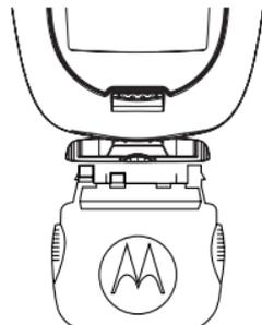
**Tip:** To remove the charger from the accessory connector: Press the buttons on the sides of the plug. Pull the plug straight out.
