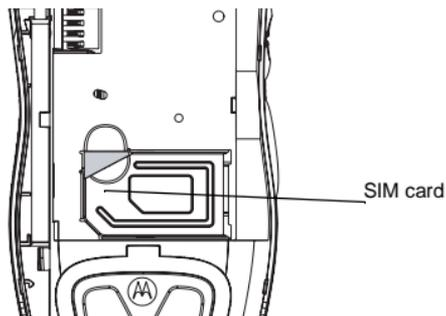
If your SIM card is not in the SIM card holder, it may be in the box your handset came in, attached to the SIM carrier. If this is the case, carefully detach your SIM card from the surrounding plastic and insert it as described in “Inserting Your SIM Card” on page 14.
