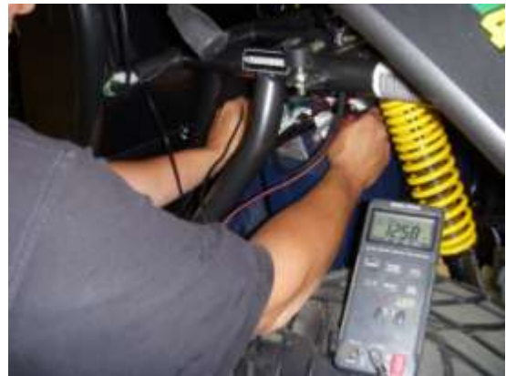
>12 volts for an individual battery
