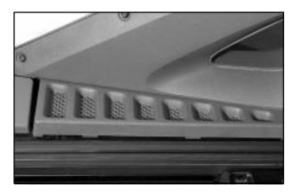
The top drain grates are located near the rear glass on both sides of the vehicle. You may need to clean the grates and drains if there seems to be blockage. But first you will have to remove the drain grates by pulling them off of the vehicle. To remove each drain grate, do the following:
