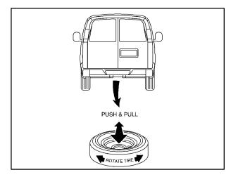
7. Make sure the tire is stored securely. Push, pull, and then try to rotate or turn the tire. If the tire moves, use the wheel wrench to tighten the cable.
