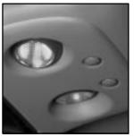
Press the button located next to each lamp to turn the lamp on. The lamps can be adjusted to point in the direction you want.
