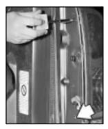
2. Remove the two rear lamp assembly screws near the tailgate latch and pull out the lamp assembly.
