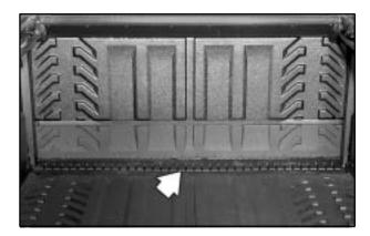
The Midgate drain grate is located near the base of the Midgate (the Midgate side facing outside). You will find a removable drain grate covering the drain.
