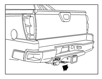
Your vehicle is equipped with the eight-wire trailer towing harness. This harness with a seven-pin universal heavy-duty trailer connector is attached to a bracket on the platform hitch.\*
