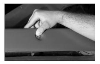
Your vehicle is equipped with Top-Box Storage units on both sides of the vehicle. The passenger side Top Box contains the tools you will need to change a flat tire.
