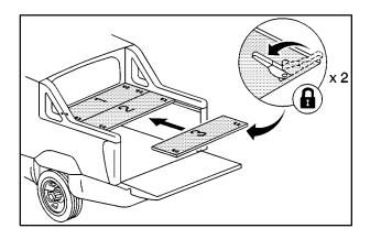
7. Push the latches away from you (start with the left latch) to lock the panel in place. You should hear a click when each latch locks correctly.
