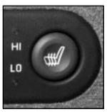
If your vehicle has this feature the button used to control the driver's side heated seat is located on the driver's side door panel. The button for the passenger's side heated seat is located on the passenger's side door panel.
