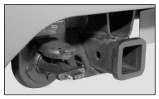
Connect the adapter with the tab (arrow) pointing towards the top. The cap on the wiring harness will lock onto the tab (arrow) and help hold the adapter in place.
