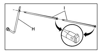
3. Attach the wheel (H) wrench and extensions (I) together.
