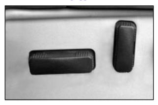
**Horizontal Control:** If your vehicle has a power seat, you can adjust it with the horizontal control located on the outboard edge of the seat(s).
