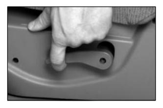
To adjust the front seatback, lift the lever. The lever is located on the outboard side of the seat cushion. Release the lever to lock the seatback where you want it. Lift the lever without pushing on the seatback and the seatback will go to an upright position.
