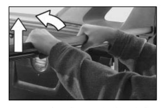
4. Remove the front rail (A) (near the midgate) by first twisting up the edge nearest you (this helps clear the midgate seals) and then pulling it out from the side rails.
