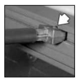
When placing the bows, locate the small notches in the side rails. These notches receive the tang on the bow ends and help the bows seat into place.
