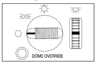
The parking/headlamp knob is located on the driver's side of the instrument panel.
