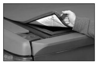
1. Starting at the rear corner of the driver's side of the vehicle, pull the loop (F) of the cover toward you and then pull up so the plastic lip (E) releases from the channel in the rear rail (D) and side rail (C).
