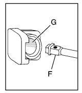
3. Insert the hoist end (open end) (F) of the extension through the hole (G) in the rear bumper.
