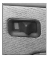
To lock the door from the inside, slide the manual lock/unlock lever rearward. To unlock the door, slide the manual lock/unlock lever forward.
