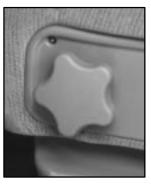
If your vehicle has a lumbar adjustment knob, you can increase or decrease lumbar support in an area of the lower seatback. The lumbar knob is located on the outboard side of the seat cushion.
