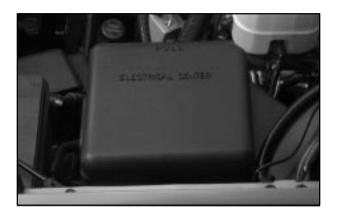
The underhood fuse block is located near the battery on the driver's side of the vehicle. Lift the cover for access to the fuse/relay block. See "Engine Compartment Overview" in the Index for more information on location.
