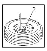
Put the tire on the ground at the rear of the vehicle with the valve stem pointed upward.
