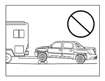
Four-wheel drive vehicles are not designed to be dolly towed.
