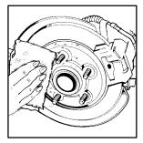
4. Remove any rust or dirt from the wheel bolts. mounting surfaces and spare wheel.
