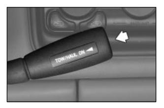
Your vehicle is equipped with a tow/haul mode. The button is located on the end of the column shift lever. You can use this feature to assist when towing or hauling a heavy load. See "Tow/Haul Mode" in the Index for more information.
