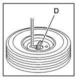
6. When the tire has been lowered, tilt the retainer (D) at the end of the cable so it can be pulled up through the wheel opening.
