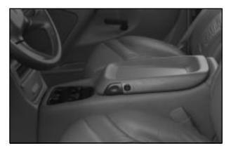
To open it, insert the console key into the lock and unlock the console. Press the button and swing the console lid open. The console has a place to store tissues, pens and a clip to hold business cards.
