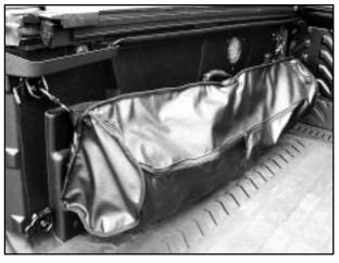
1. Attach the bag to the cargo tie downs as shown. Unzip the top of the storage bag so it will be ready when you need to stow the tonneau cover.
