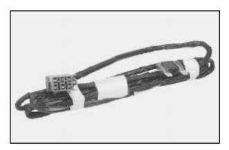
This harness is included with the heavy-duty trailer wiring package. The harness is for an electric trailer brake controller and includes a trailer battery feed fuse. This harness and fuse should be installed by your dealer or a qualified service center.
