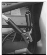
8. Now connect the black negative (-) cable to the negative (-) terminal of the good battery. Use a remote negative (-) terminal if the vehicle has one. Your vehicle's remote negative (-) terminal is marked "GND."
