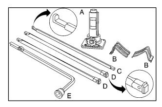
The tools you'll be using include the jack (A), the wheel blocks (B), the jack handle (C), the jack handle extensions (D), and the wheel wrench (E).
