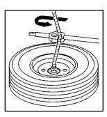
5. The wheel wrench has a hook that allows you to pull the hoist cable towards you to assist in reaching the spare tire.
