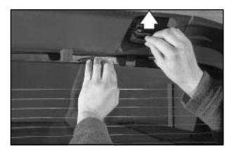
6. Use one hand to push the rear glass flat against the window frame and with your free hand push each latch lever up until it locks. You should hear a click when each latch lever locks correctly.
