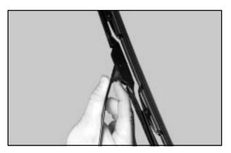
Windshield wiper blades should be inspected at least twice a year for wear and cracking. See "Wiper Blade Check" in the Index for more information. Replacement blades come in different types and are removed in different ways. For proper type and length, see "Normal Maintenance Replacement Parts" in the Index. Here's how to remove the Shephard's Hook type.
