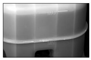
You can check the brake fluid without taking off the cap. Just look at the brake fluid reservoir. The fluid level should be above MIN. If it isn't, have your brake system checked to see if there is a leak.
