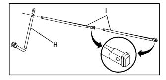
2. Assemble the wheel wrench (H) and the two jack handle extensions (I) as shown.
