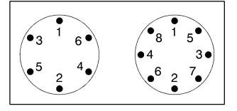
7. Tighten the nuts firmly in a crisscross sequence as shown by turning the wheel wrench clockwise.
