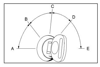
A (ACCESSORY): This position allows you to use things like the radio, power windows and the windshield wipers when the engine is off. Push in the key and turn it toward you.
