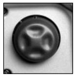
If you have power lumbar adjustment, you can increase or decrease lumbar support in the lower seatback. The control is located on the outboard side of the seat cushion.
