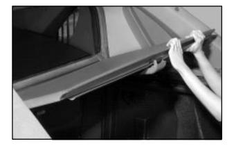
2. Starting with cargo panel 1, place the latches in the open (unlocked) position. Place cargo panel 1 on the cargo area rails while holding the back of the cargo panel up.
