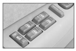
The controls for the power windows are located on each of the side doors in the front and rear.
