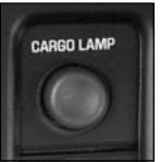
Press this button, located on the instrument panel to turn the cargo lamps on. Press the button again to turn it off.
