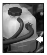
When the engine is cold, the coolant level should be at or above the FILL COLD mark. If it isn't, you may have a leak in the radiator hoses. heater hoses, radiator, water pump or somewhere else in the cooling system.
