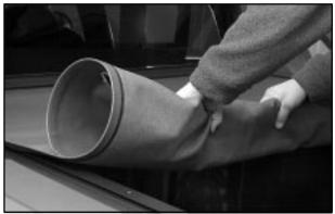
3. Roll the cover toward the front of the vehicle (the plastic lip will release from the siderails as you roll the cover forward). When you reach the front rail (A), pull the cover out from the front rail and roll up the rest of the cover.
