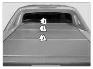
Before removing the cargo panel(s), notice the numbers embossed on the upper center portion of each panel. The panels are labeled 1, 2 and 3. There are also numbered labels on the bottom of the panels. The numbers on the top and bottom of the panels will be used as reference when removing, storing and reinstalling the panels.
