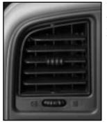
Your vehicle has air outlets in the center and on the sides of the instrument panel.
