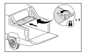
3. Push both left latches away from you to lock the latches (remember that there are two latches on each side for panel 1). You should hear a click when each latch locks correctly. Lock the remaining two right latches on panel 1.
