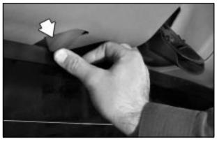
3. While holding the rear glass in place, press the glass-catch release button and pull the top of the rear glass toward you using the grab handle(s) (B) located at the top of the rear glass.
