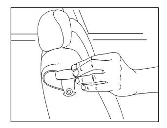
1. Remove the guide from the storage clip on the side of the rear seatback.
