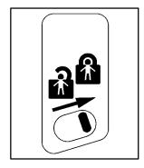
You will find a security lock lever on the inside edge of each rear door. Your vehicle may be equipped with one of the two labels shown.
