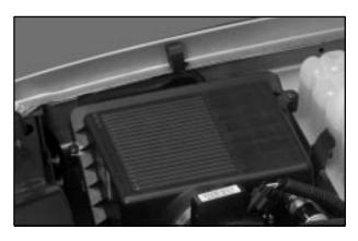
Your engine air cleaner/filter is located on the front corner of the engine compartment on the passenger's side of the vehicle. See "Engine Compartment Overview" in the Index for more information on location.
