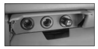
With accessory power outlets you can power auxiliary electrical equipment such as a cellular telephone or CB radio.
