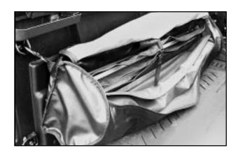
5. Stow both bows and the front and rear rails in the storage bag as shown. When all components of the tonneau cover are secured in the bag properly, zip the bag shut.
