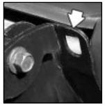
An anchor loop bracket for a top strap is located on the back of the rear seat frame above the floor for each rear seating position. In order to get to the brackets, you'll have to fold the rear seatback(s).
