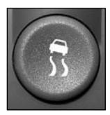
To turn the system on or off press the TAS on/off button located to the left of the of the steering wheel on the instrument panel. If you used the button to turn the system off, the TRACTION OFF light will come on and stay on.
