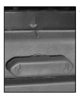
5. Be sure to align the rear glass side-to-side using the alignment arrows (G) as shown in the picture.
