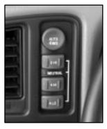
The transfer case switches are located to the left of the instrument panel cluster.
