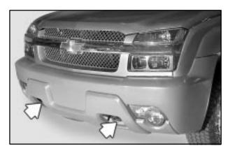
Your vehicle is equipped with recovery hooks. The hooks are provided at the front of your vehicle. You may need to use them if you're stuck off-road and need to be pulled to some place where you can continue driving.
