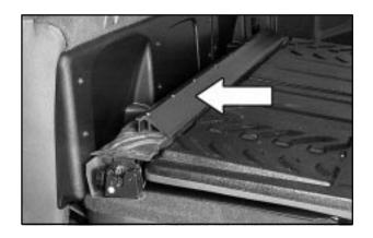
If you lower the Midgate with the rear glass in the stored position, you will notice that the entire crossbar (the bar with the release handle) will lower with the Midgate.
