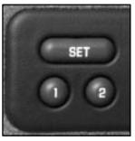
The memory function recalls the driver's seat cushion and recliner positions. The buttons are located on the driver's side door panel.
