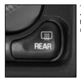
To turn on the rear window defogger, press this button located below the mode knob.
