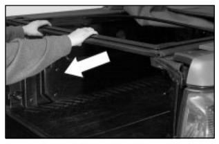
1. Remove the rear rail (D) by pulling it straight out from the side rails. Set the rail aside.
