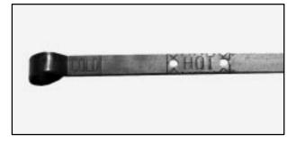
3. If the fluid level is in the acceptable range, push the dipstick back in all the way; then flip the handle down to lock the dipstick in place.
