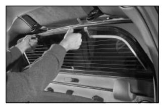
4. With the rear glass tilted at an angle, place the bottom edge in the lower channel of the window frame applying a slight downward pressure and then push the rear glass flat against the window frame. Use the grab handles at the top of the rear glass to assist you.
