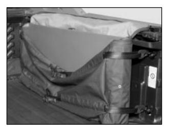
2. Starting with cargo panel 1 (the panel with four latches) load the cargo panel with latches facing outboard (side of panel with no latches should be facing you as you load the panel).
