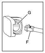
4. Insert the hoist end (F) through the hole (G) in the rear bumper and into the hoist shaft.
