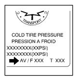
The front axle reserve capacity for your vehicle can be found in the lower right corner of the tire/certification label.
