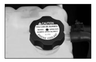
5. Then replace the pressure cap. Be sure the pressure cap is hand-tight.
