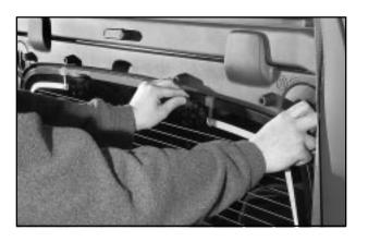
6. Turn both glass lock knobs (D), located at both top corners of the storage pocket, to the locked position. You may need to push the corner of the rear glass to allow the lock knob to engage more easily.
